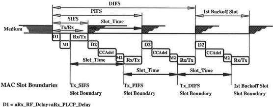
D1 = aRx\_RF\_Delay+aRx\_PLCP\_Delay D2 = D1 + Air\_Propagation\_Time RxTx = aRxTx\_Turnaround\_Time M1,M2 = aMAC\_Prx\_Time CCAdel = aCCA\_Asmnt\_Time
