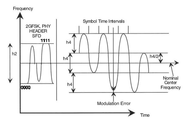
Figure A, 4 Level GFSK Transmit Modulation
