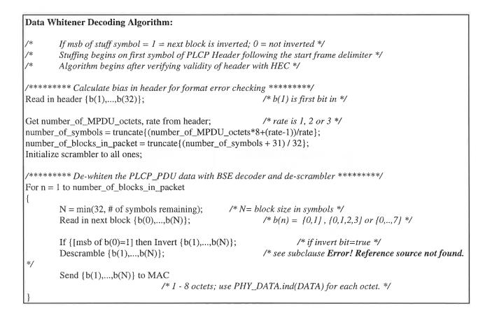
Figure C, Data Whitener Decoding Procedure
