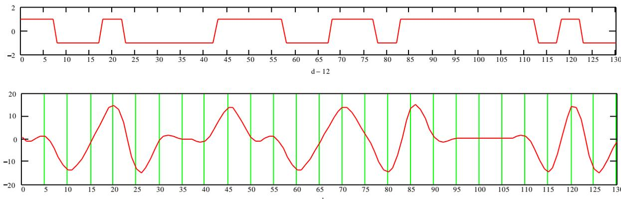
**Figure 1 Data stream and associated 3-level analog waveform**
