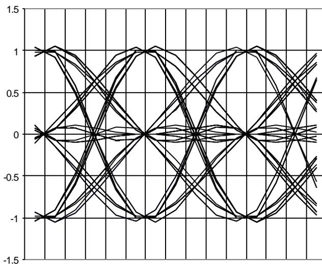
**Figure 2 Simulation “eye” diagram for 3-level modulation**
