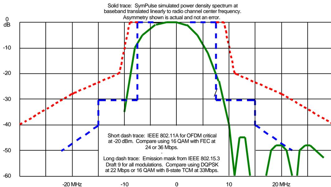
**Figure 4.** Spectrum of Fig.3 shown against the IEEE P802.11b and 802.15.3 masks
