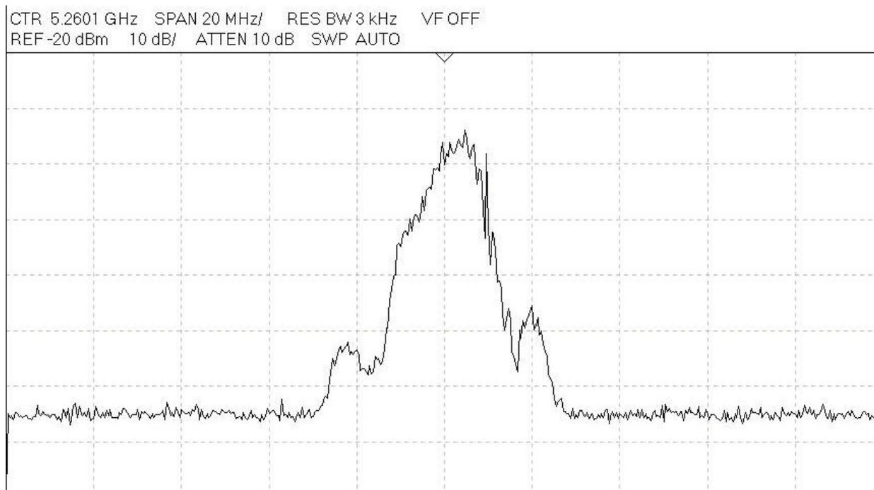
**Figure 7 Sym-pulse power density spectrum after translation to 5.26 GHz**
