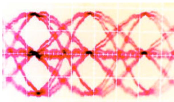
Figure 6 Measured eye diagram at baseband
