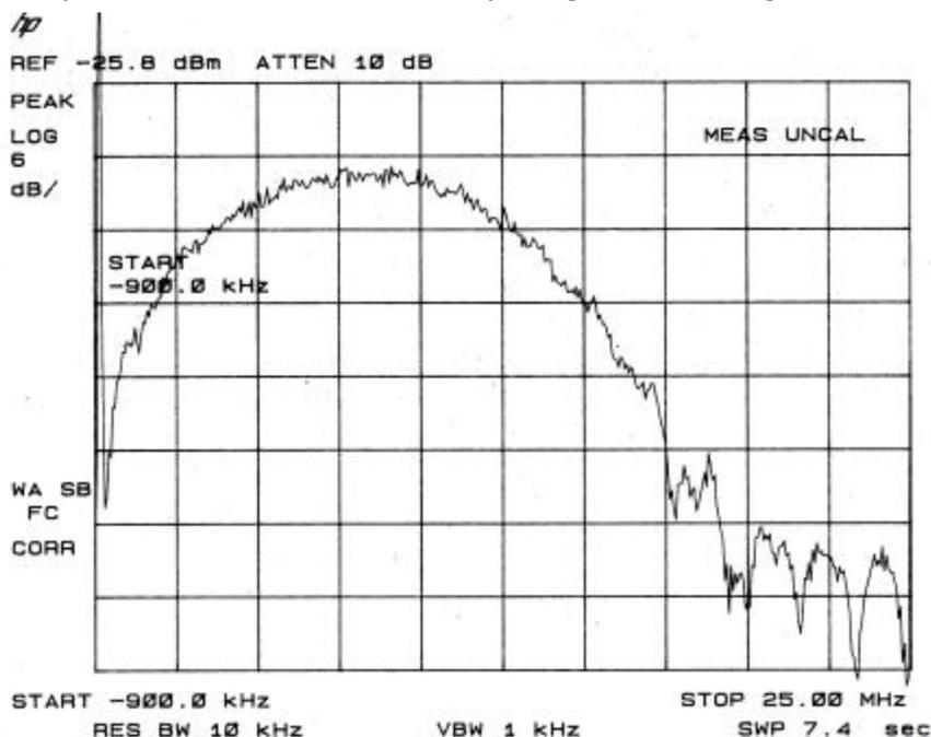
Figure 5 Measured basband spectrum for a random data stream with sym-pulse.
