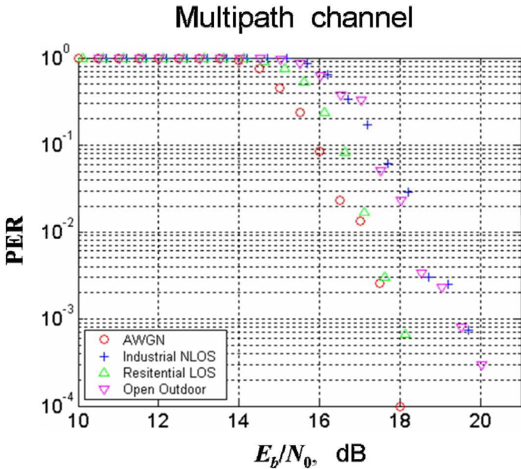
Fig. 7.2. Performance of the system in multipath channels (PER).
