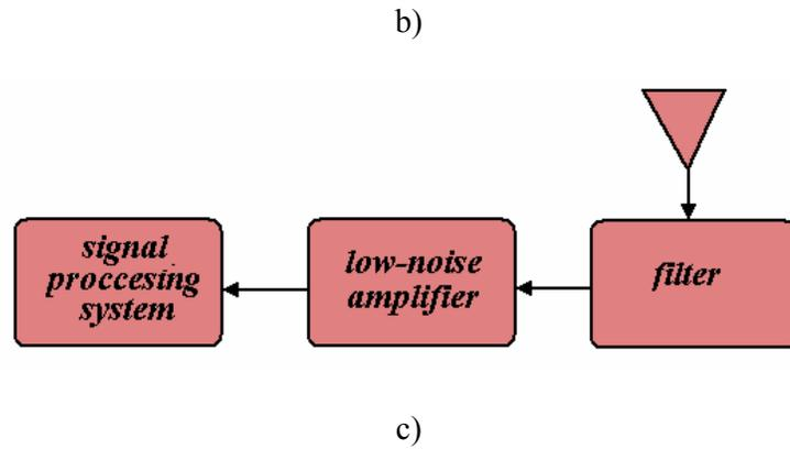
Fig. 2.1.1. Block-diagram of direct chaotic communication system: (a) transmitter with external modulation; (b) transmitter with internal modulation; (c) receiver.
