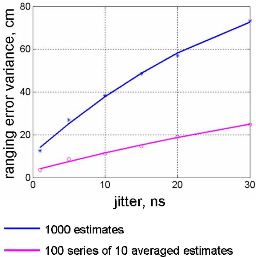
Fig. 13.3.3. Ranging error variance vs. jitter time.
