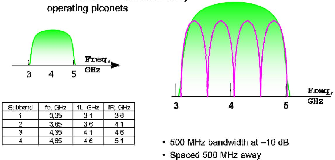
Fig. 6.2.1. Subbands for simultaneously operating piconets
