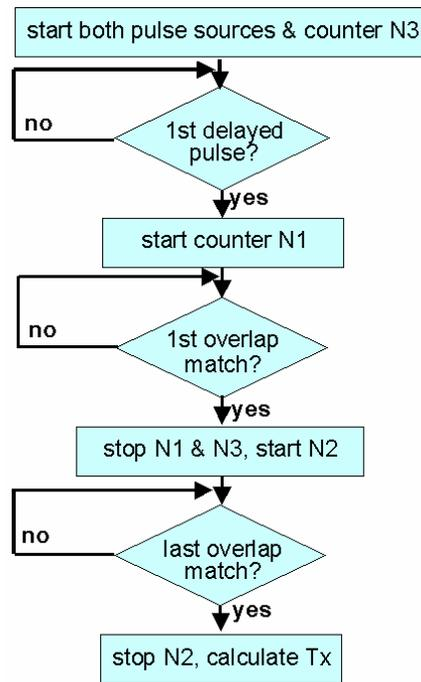
Fig. 13.2.2. Structure of the ranging algorithm.
