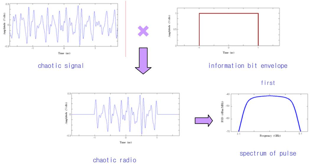
Fig. 2.3.1. Chaotic radio pulse and its features
