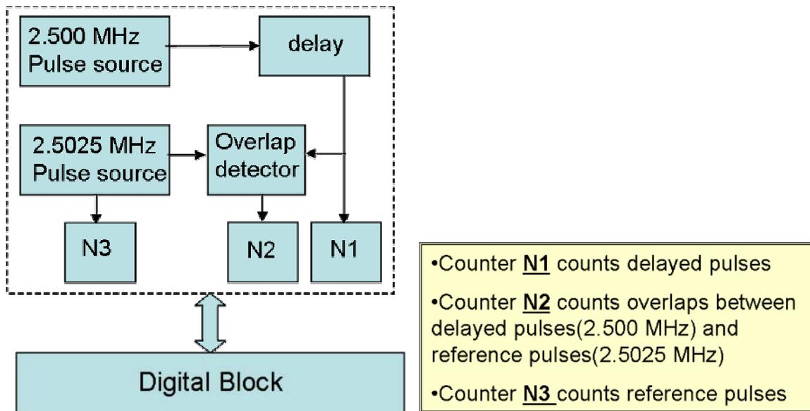
Fig. 13.2.1. Block diagram of the proposed ranging method.
