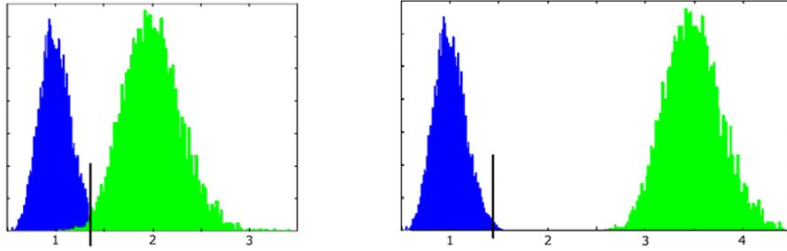
Fig 2.5.4. Distributions of energy per bit for same-duration pulses at different distances: (a) maximum distance; (b) less distance. Constant threshold is shown.
