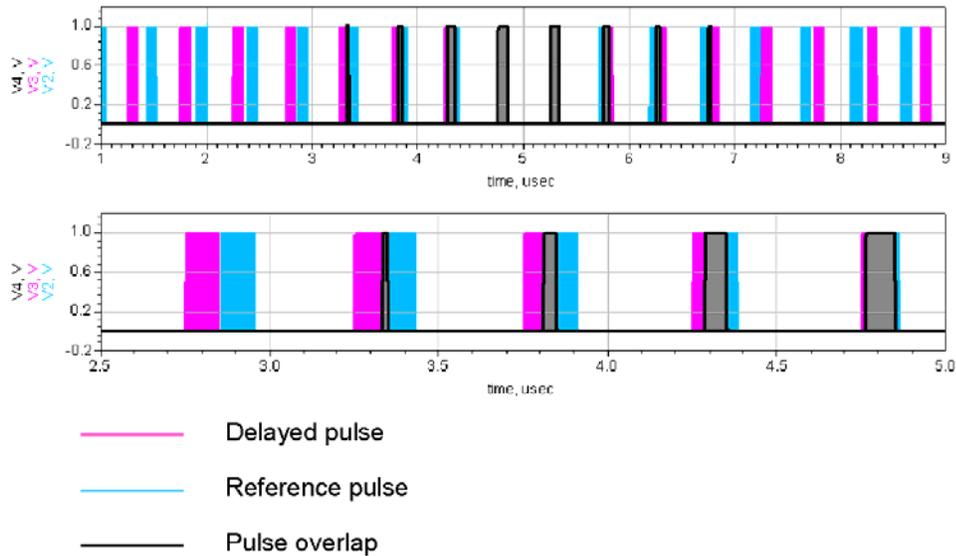
Fig. 13.3.2. Overlapping of reference and probing signal pulses.
