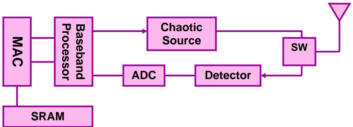
Fig. 2.7.1. Transceiver architecture
