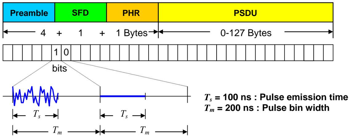
Fig. 2.6.1. Frame structure
