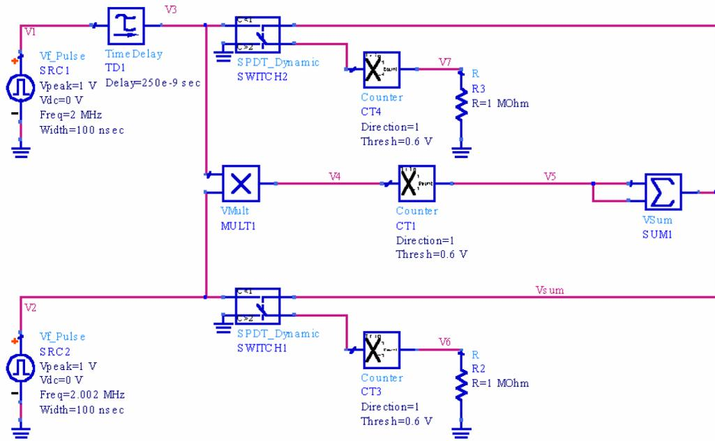
Fig. 13.3.1. Simulation circuit in ADS.
