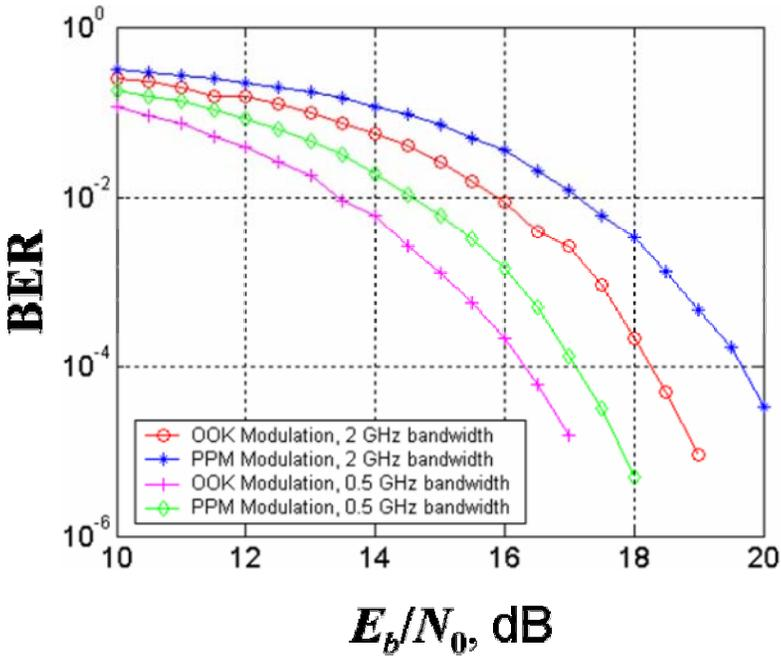
Fig. 7.1. BER (bit error ratio) as a function of the ratio of energy-per-bit to spectral density of noise in the channel.
