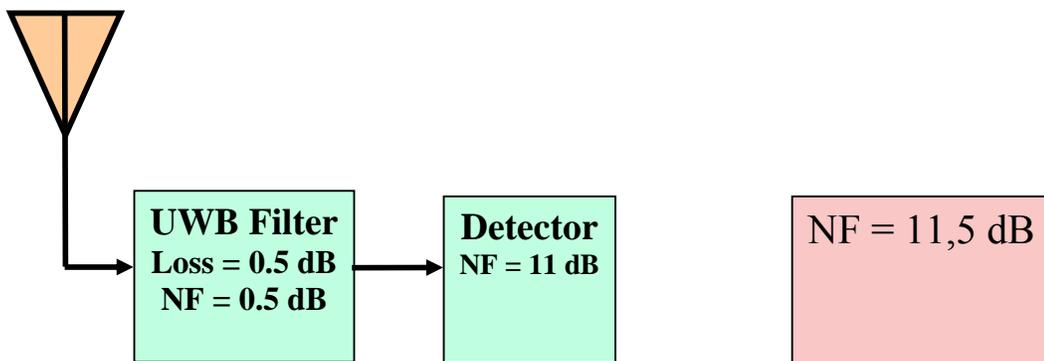
Fig. 2.7.1. Radio receiver. Example 1.
