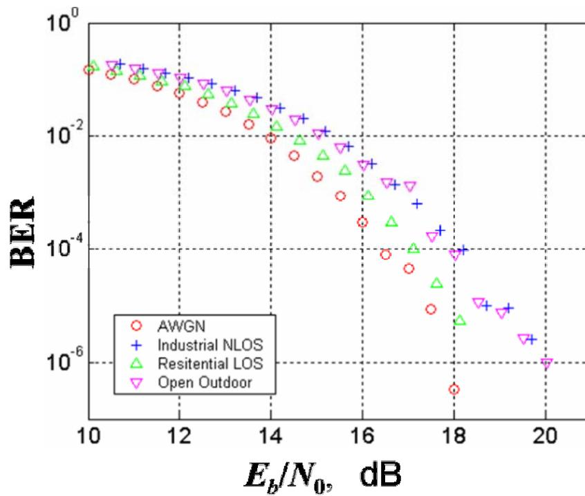
Fig. 7.2. Performance of the system in multipath channels (BER).
