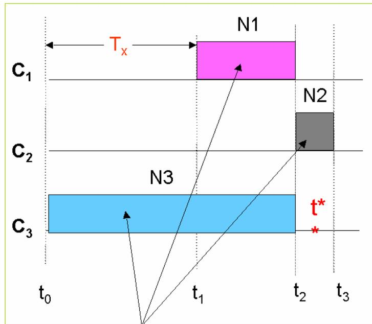
**Operation time of counters C1,C2,C3** Fig. 13.2.3. Time diagrams describing the logics of operation of counters C1-C3.
