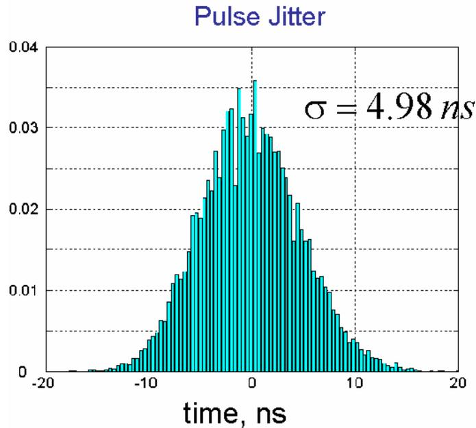
Fig. 13.3.4. The distribution of pulse front detection time
