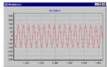
Figure 3. Parts of the payload during a frequency offset measurement where each 1 and 0 in the received payload is over-sampled 9 times. The used payload is 01010101<sup>1</sup>.
