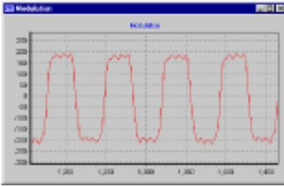
Figure 4. Parts of the Payload during a transmitter deviation measurement. The used payload is 00001111<sup>1</sup>.
