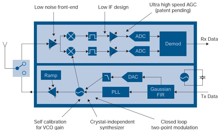
*The Philsar PH2401 single-chip radio provides Bluetooth-specific architecture.*
