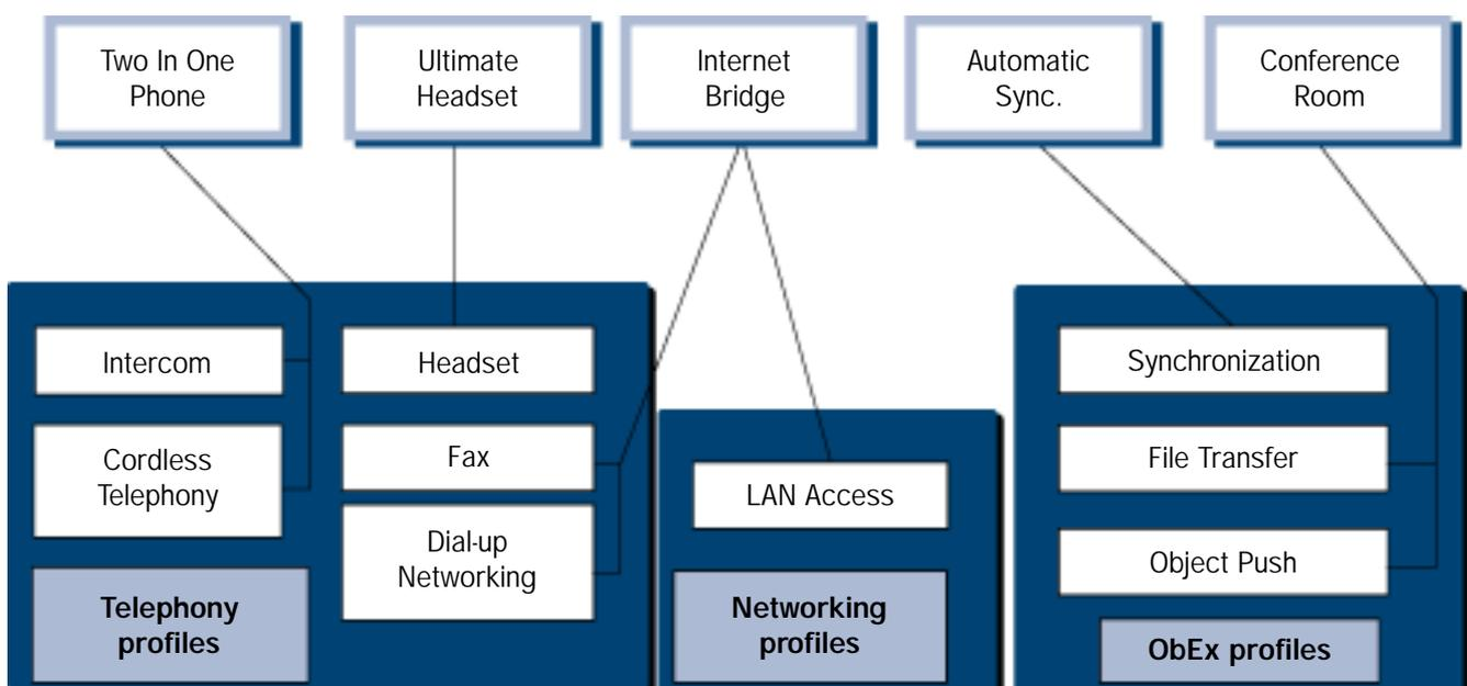
Fig. 1 The relationship between usage models and profiles.
