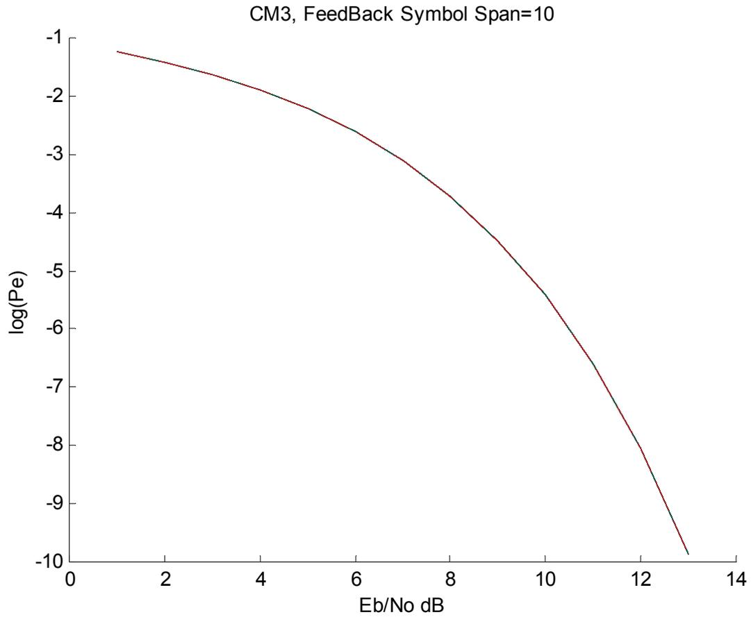
2.8.24 10 Symbol Span Equalizer Low Band (1/57e6 symbol duration)
