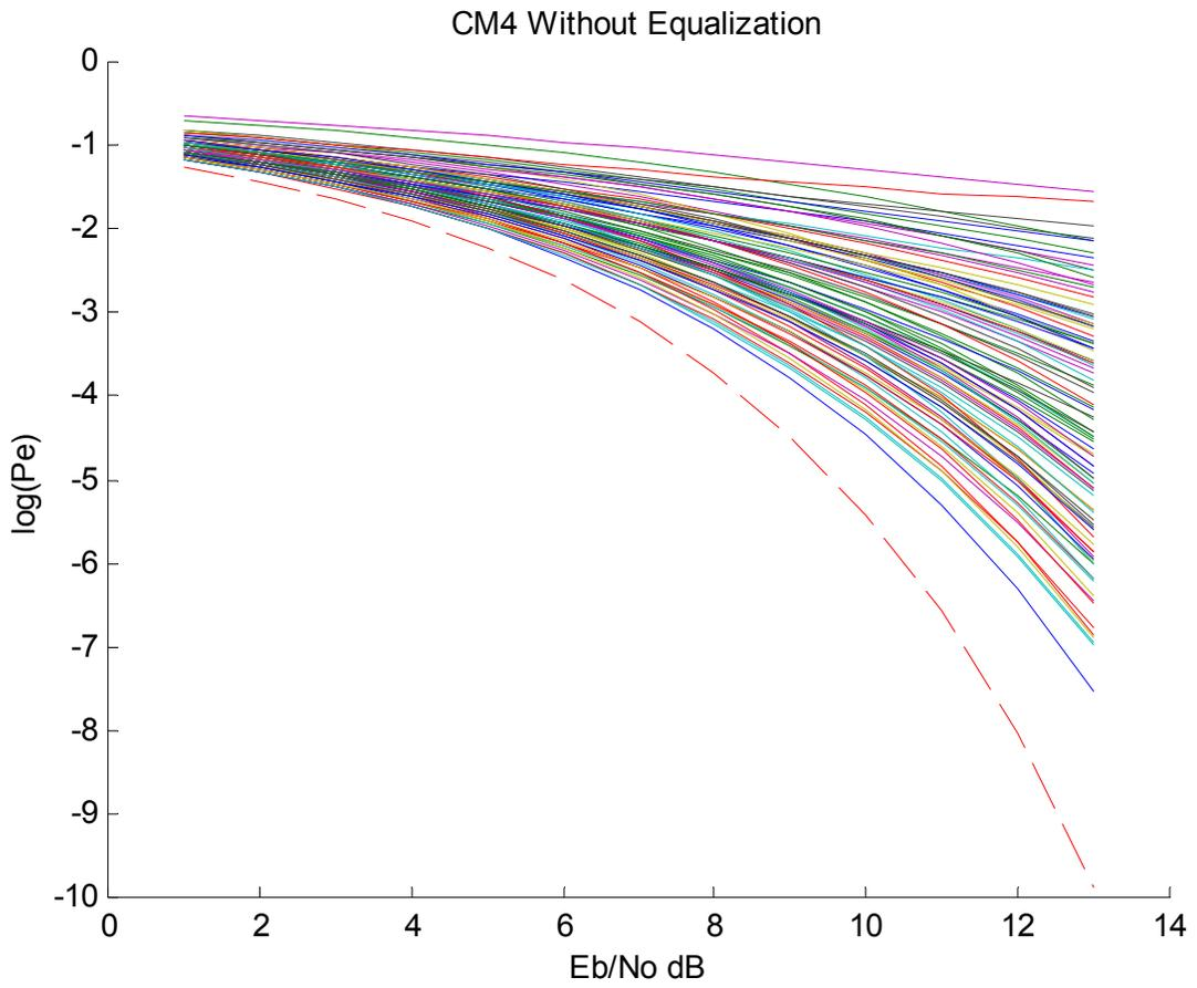
2.8.9 5 Symbol Span Equalizer High Band (1/114e6 symbol duration)
