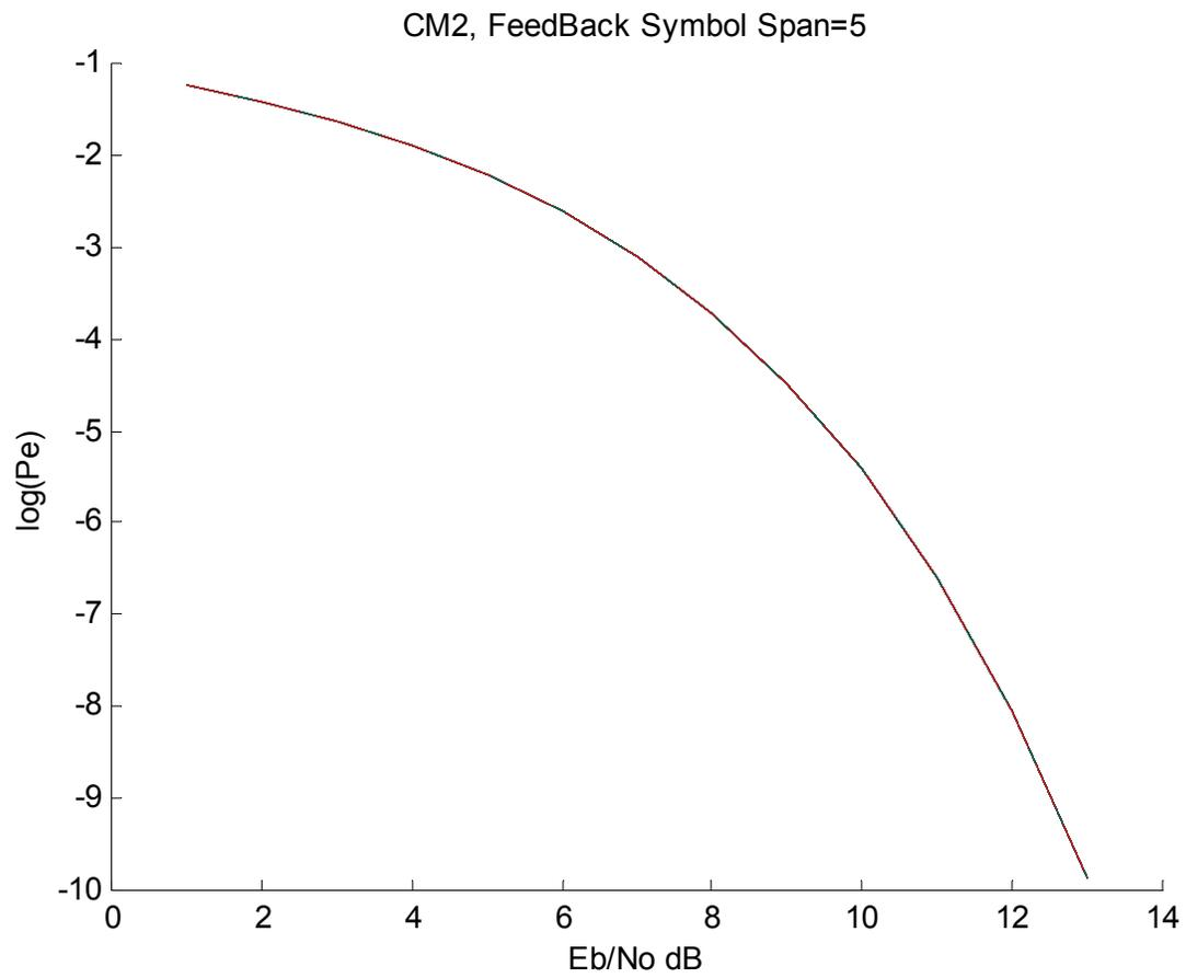
2.8.15 5 Symbol Span Equalizer Low Band (1/57e6 symbol duration)
