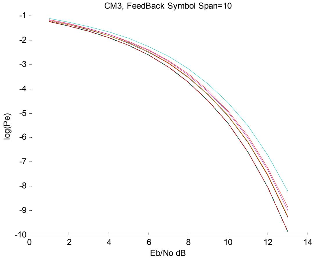
2.8.20 10 Symbol Span Equalizer High Band (1/114e6 symbol duration)
