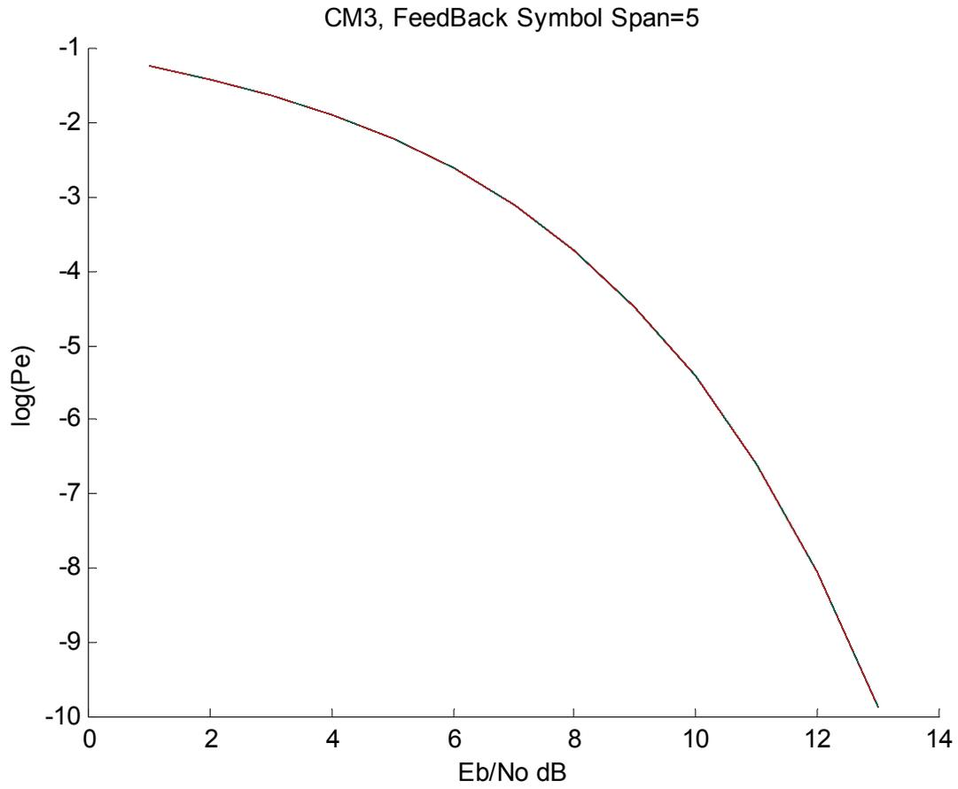
2.8.16 5 Symbol Span Equalizer Low Band (1/57e6 symbol duration)
