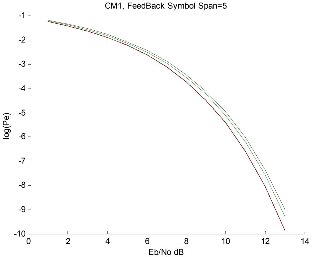
2.8.10 5 Symbol Span Equalizer High Band (1/114e6 symbol duration)
