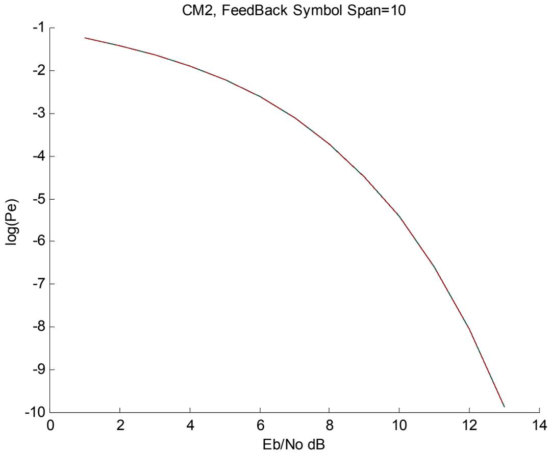
2.8.19 10 Symbol Span Equalizer High Band (1/114e6 symbol duration)
