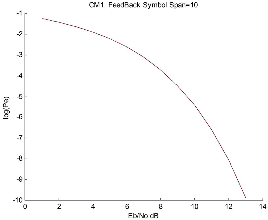
2.8.22 10 Symbol Span Equalizer Low Band (1/57e6 symbol duration)
