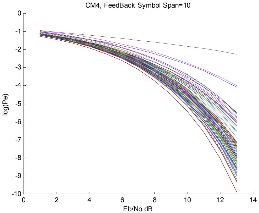
2.8.21 10 Symbol Span Equalizer Low Band (1/57e6 symbol duration)
