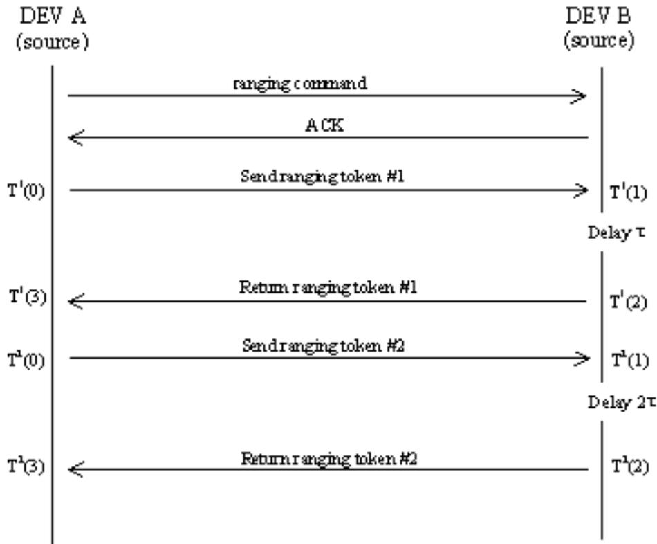
Figure 1 - MSC for ranging token exchange
