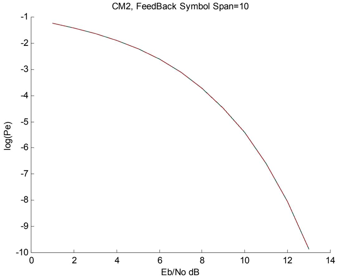
2.8.23 10 Symbol Span Equalizer Low Band (1/57e6 symbol duration)
