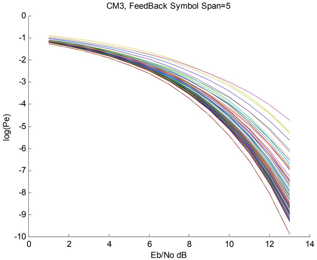
2.8.12 5 Symbol Span Equalizer High Band (1/114e6 symbol duration)
