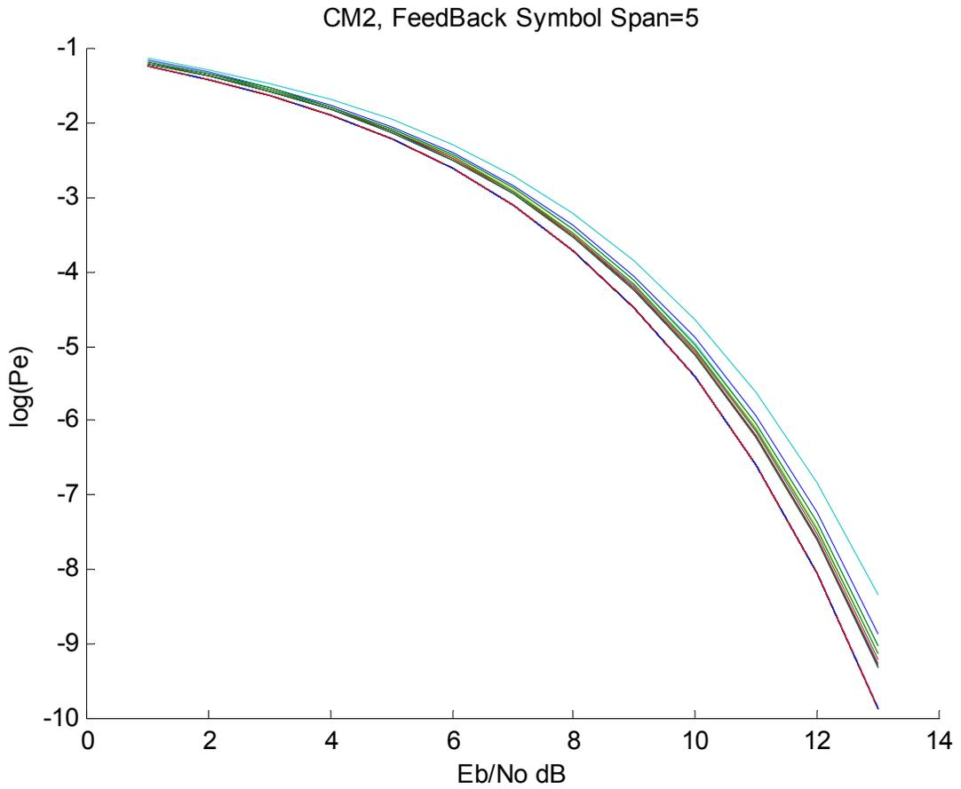
2.8.11 5 Symbol Span Equalizer High Band (1/114e6 symbol duration)
