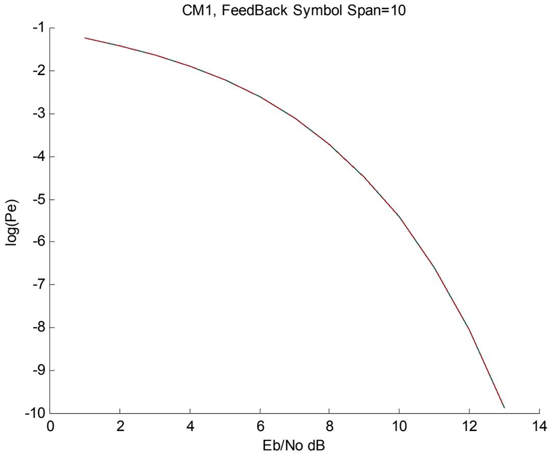
2.8.18 10 Symbol Span Equalizer High Band (1/114e6 symbol duration)
