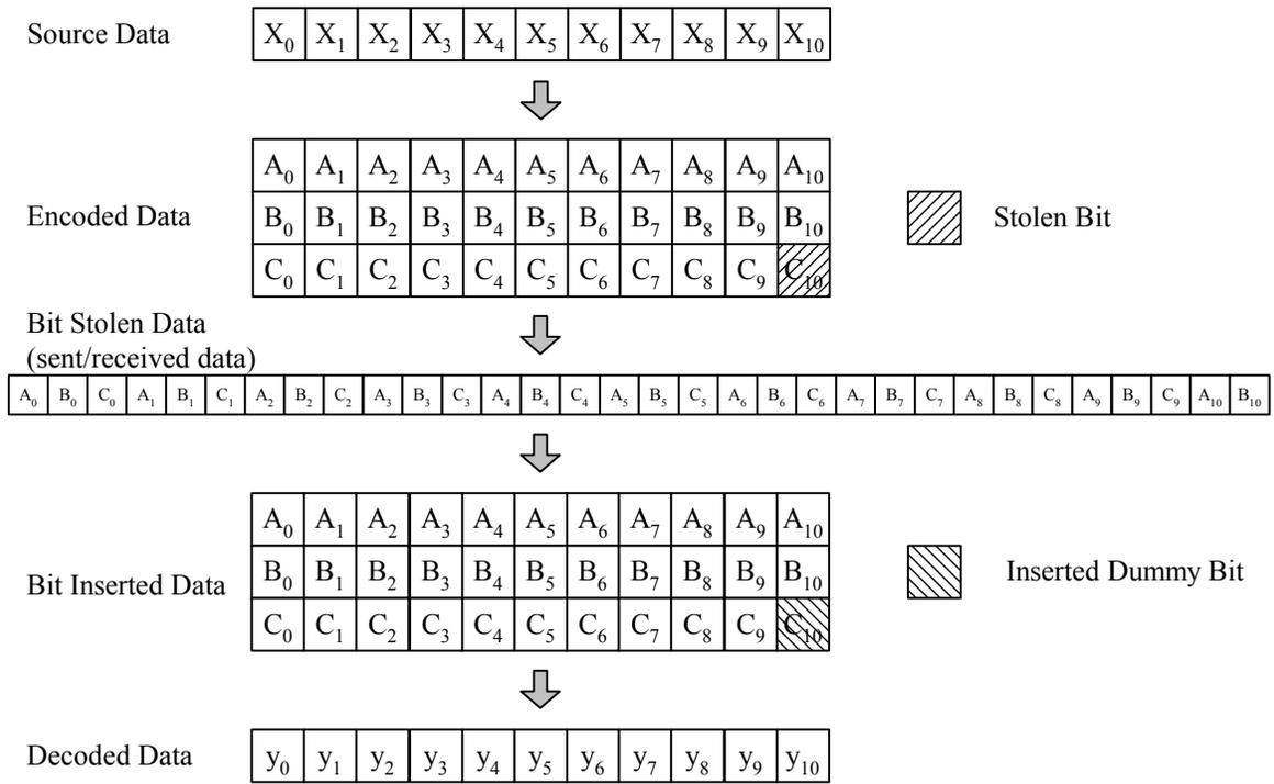
**Figure 8 – An example of the bit-stealing and bit-insertion procedure (R = 11/32)**
