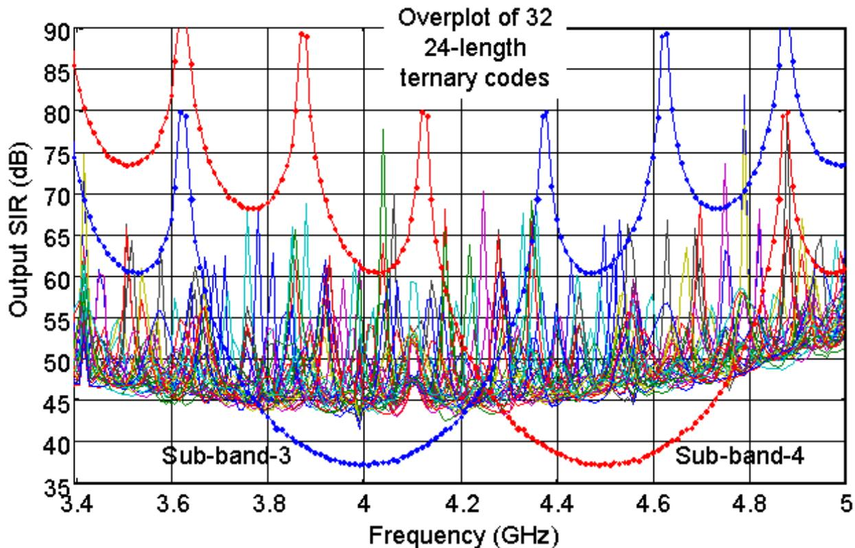
Figure 3. Interference rejection for DSSS-UWB and pulsed sub-band systems showing the combined effects of processing gain and pulse shape filtering.
