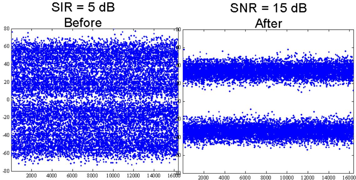
Figure 4. Eye pattern (left) of 15 dB SNR signal with NBI giving 5 dB SIR, and (right) eye pattern after DSP removal of NBI showing 15 dB SNR.
