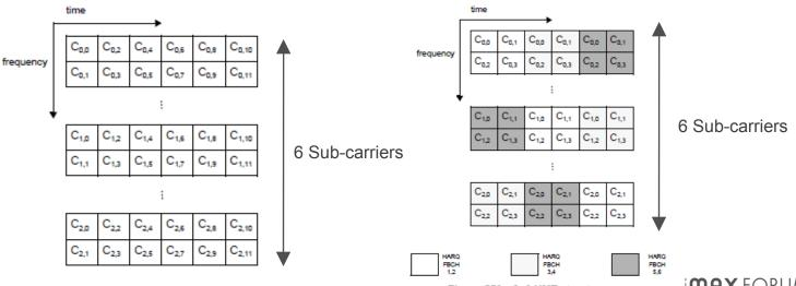
Figure 555—PFBCH comprised of three distributed 2x6 UL FMTs
