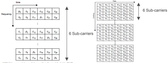
Figure 557—SFBCH comprising of three distributed 2x6 UL FMTs
