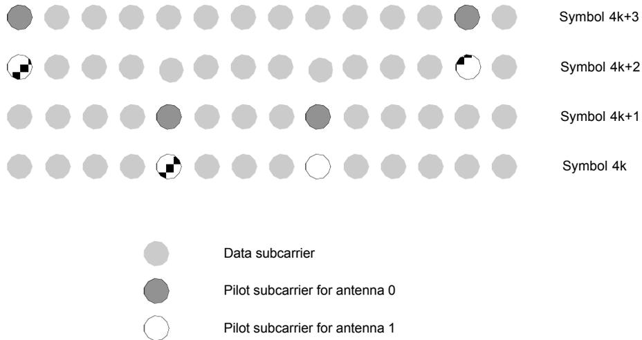
**Figure 245 – Cluster structure for STC PUSC using 2 Antennas**
