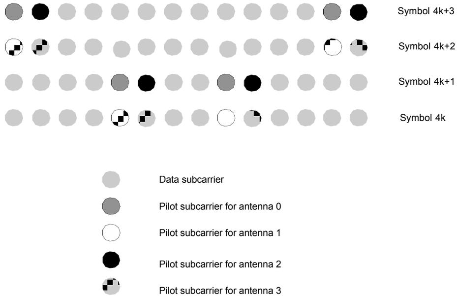
**Figure 245 – Cluster structure for STC PUSC using 4 Antennas**
