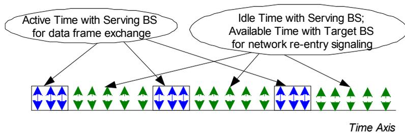
Figure-1: Low Latency Handover Principle
