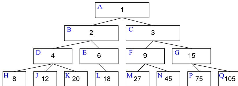
**Figure 5: CIDs for MS-BS/RS tree assuming Figure 1 topology. The root node, A, is the BS; all other nodes are RS.**
