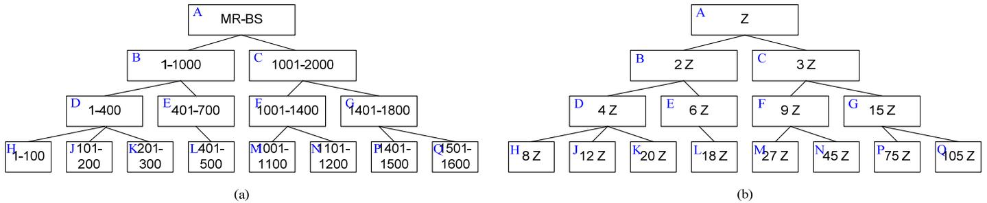
**Figure 6.3.1.3.Y: CID range allocation example, (a) contiguous integer block, (b) prime factorization method.**
