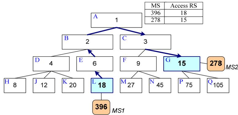
Figure 6: An example of relay path configuration using prime factoring method.
