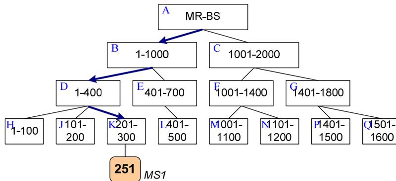
Figure 8: An example of relay path configuration using contiguous integer method.
