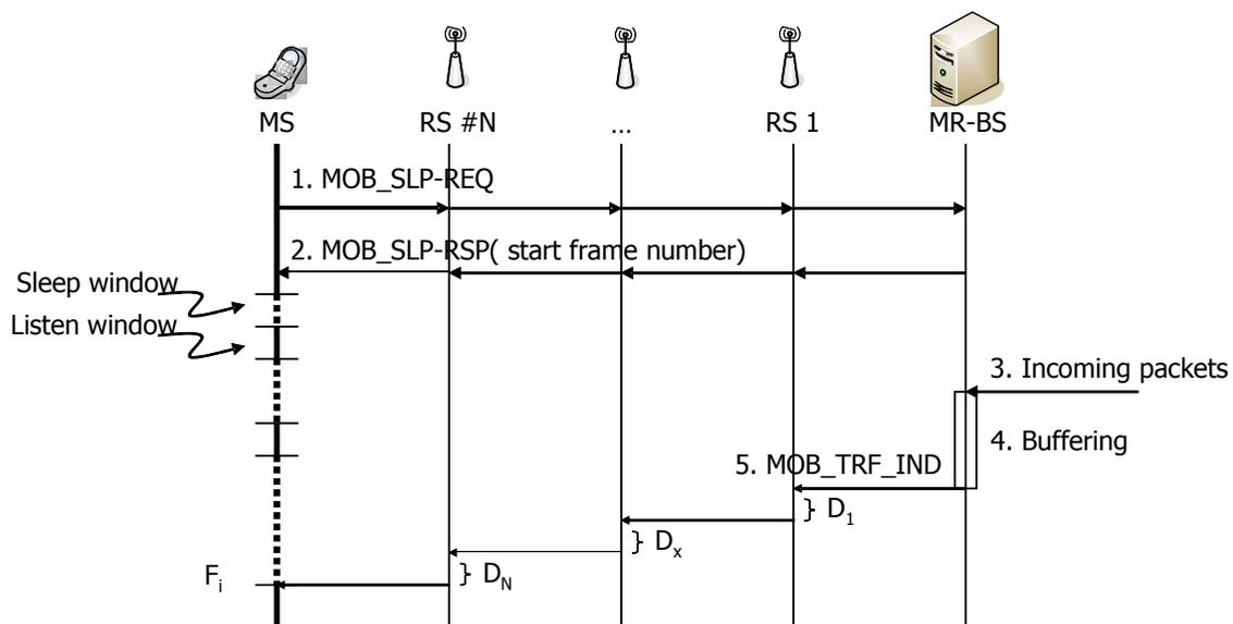
Figure 1. MS sleep mode support for centralized scheduling
