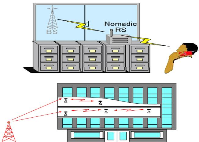
Figure 2 Examples of In-building Coverage Usage Model
