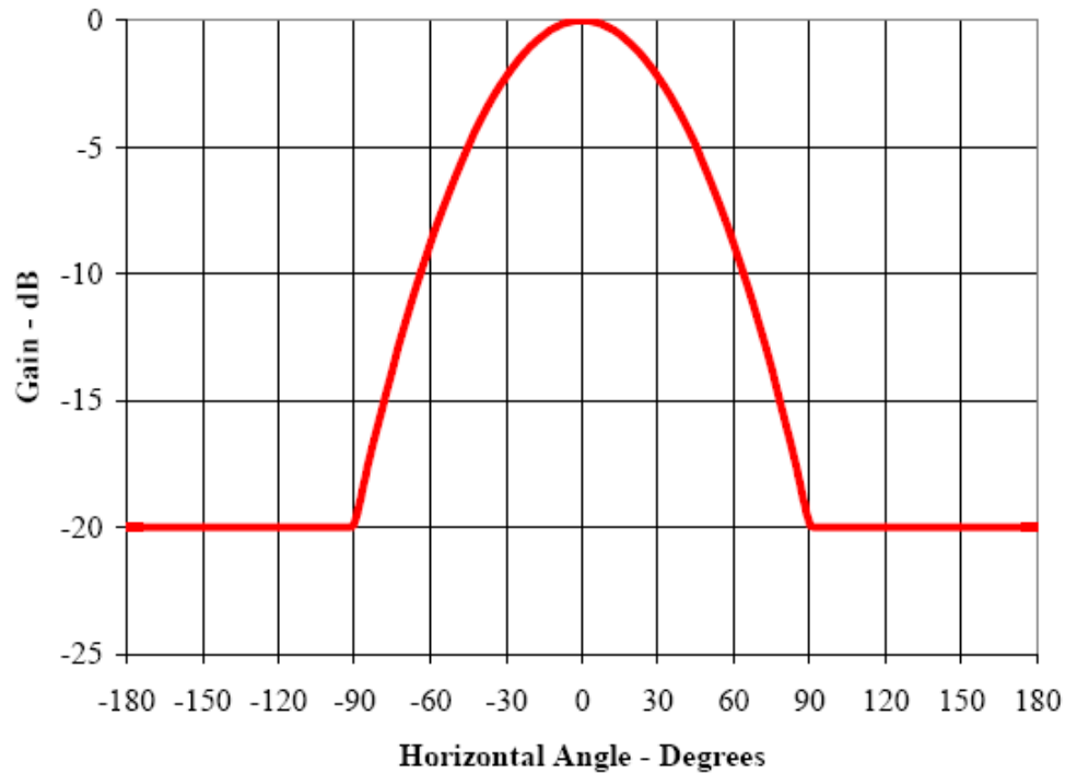
Figure 2: Antenna Pattern for 3-Sector Cells
