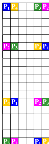
Figure 48: Pilot Pattern for four stream pilots, P_k denotes pilot for stream k .
