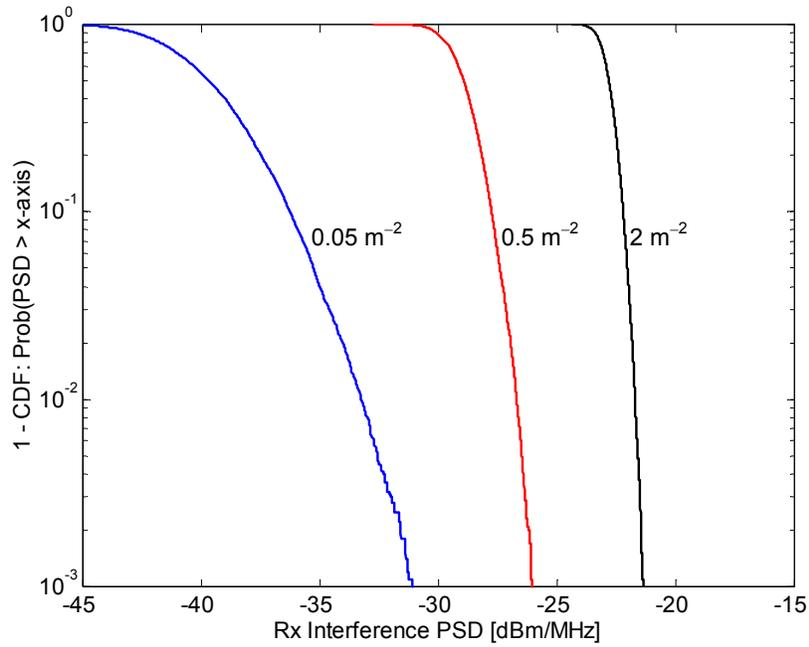
**Figure A7.3. Statistics for aggregate interference PSD at 2 GHz. EIRP of 0 dBm/MHz, minimum distance of 1 m, activity factor of 100%.**
