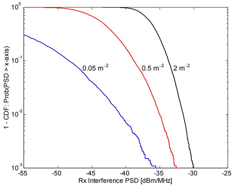
**Figure A7.4. Statistics for aggregate interference PSD at 2 GHz. EIRP of 0 dBm/MHz, minimum distance of 1 m, activity factor of 5%.**
