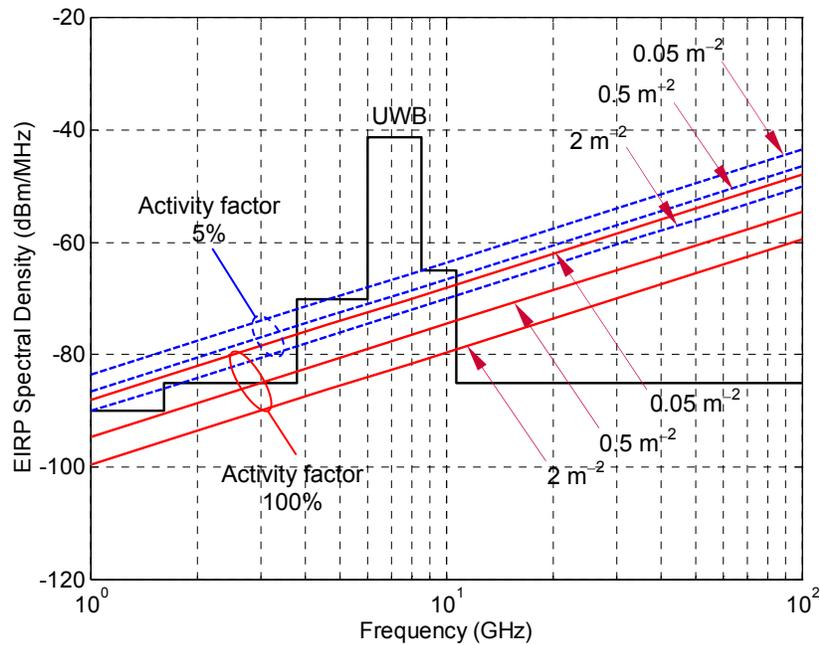
Figure A7.9. EIRP spectral density limits for low-power devices, such that resulting aggregate interference exceeds 5% of thermal noise with a probability of 0.1%. Minimum distance from measurement point of 2 m.
