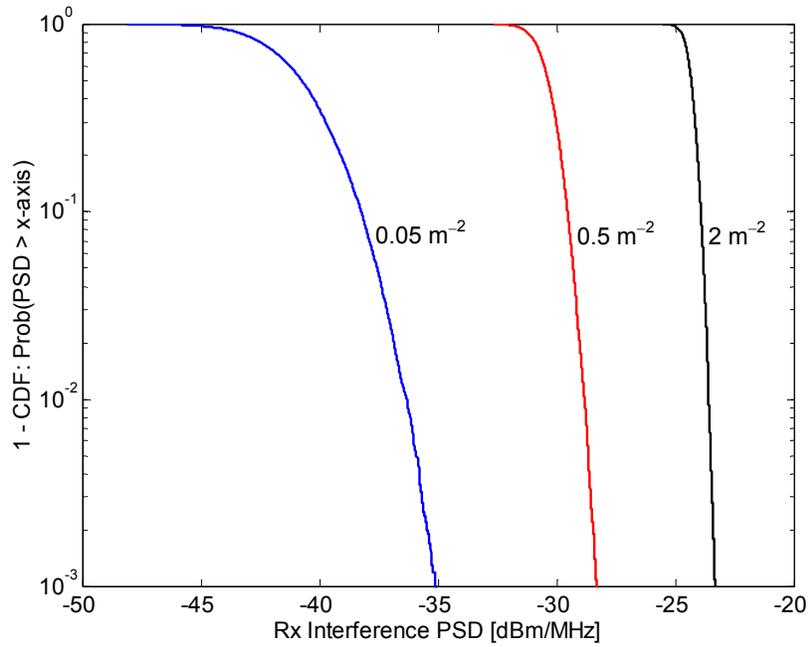
Figure A7.5. Statistics for aggregate interference PSD at 2 GHz. EIRP of 0 dBm/MHz, minimum distance of 2 m, activity factor of 100%.
