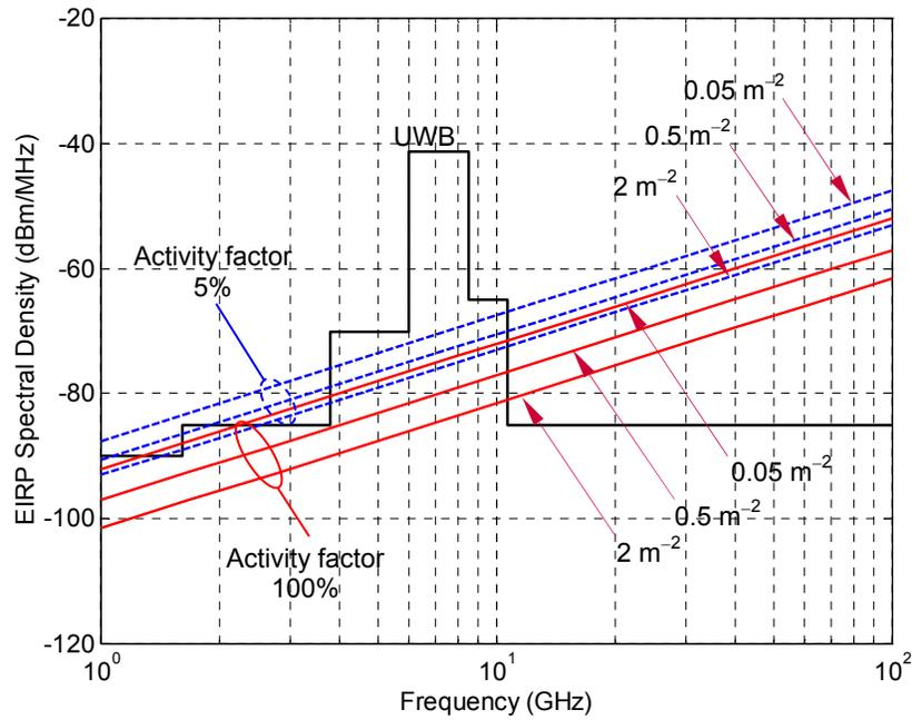
Figure A7.8. EIRP spectral density limits for low-power devices, such that resulting aggregate interference exceeds 5% of thermal noise with a probability of 0.1%. Minimum distance from measurement point of 1 m.
