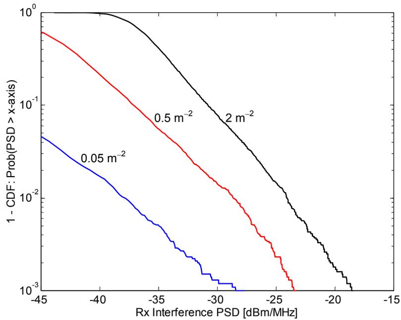
Figure A7.2. Statistics for aggregate interference PSD at 2 GHz. EIRP of 0 dBm/MHz, minimum distance of 0.15 m, activity factor of 5%.
