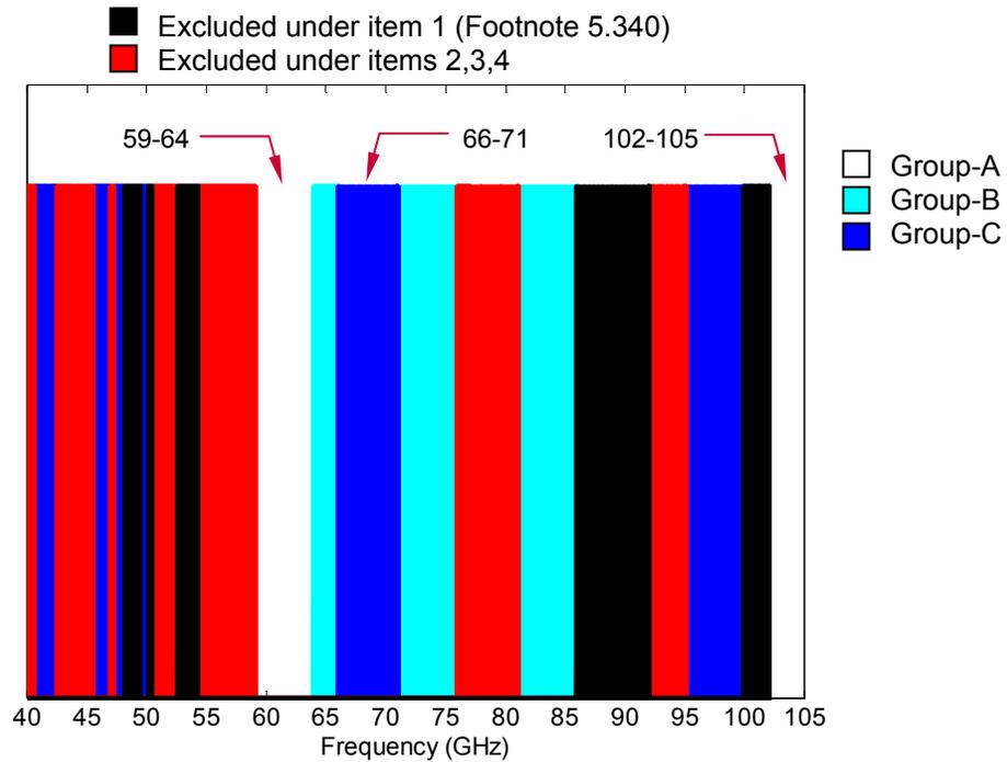
**Figure 6. Spectrum potentially available for future applications in the 40–105 GHz band.**
