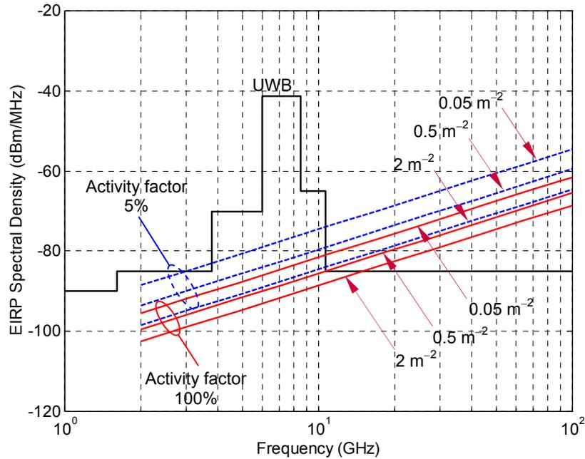
**Figure A7.7. EIRP spectral density limits for low-power devices, such that resulting aggregate interference exceeds 5% of thermal noise with a probability of 0.1%. Minimum distance from measurement point of 0.15 m.**
