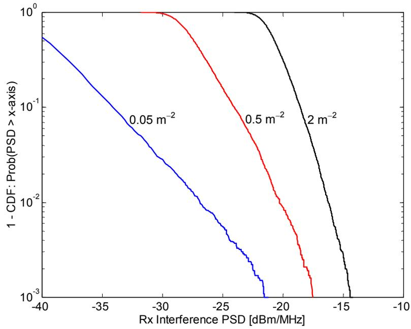
Figure A7.1. Statistics for aggregate interference PSD at 2 GHz. EIRP of 0 dBm/MHz, minimum distance of 0.15 m, activity factor of 100%.
