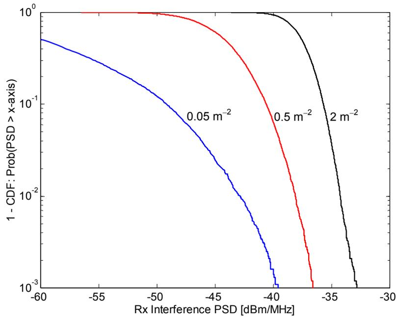
Figure A7.6. Statistics for aggregate interference PSD at 2 GHz. EIRP of 0 dBm/MHz, minimum distance of 2 m, activity factor of 5%.
