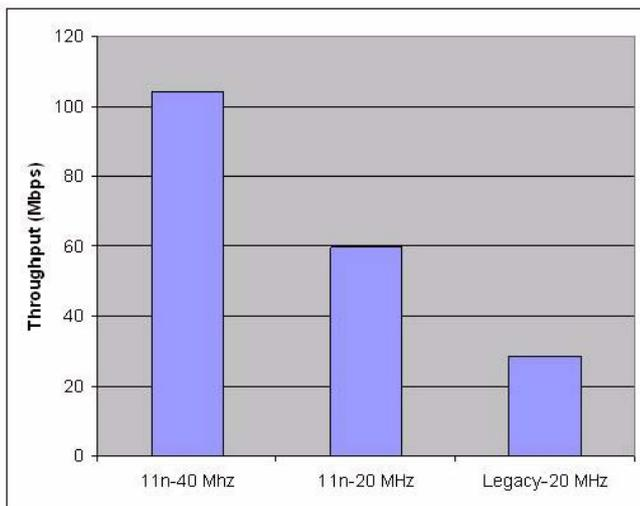
Fig. 3. Maximum throughput of 20/40 MHz BSS and 20 MHz legacy BSS.
