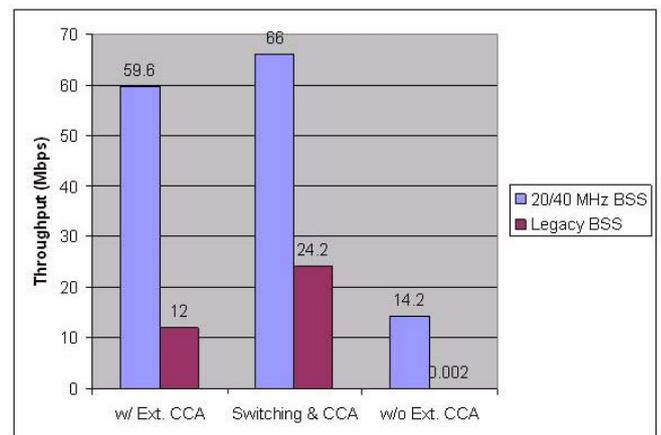
Fig. 5. Throughput of overlapping BSSs when channel switching is used.
