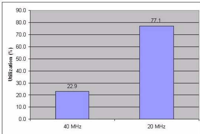
Fig. 6. Utilization of 20/40 MHz BSS when channel switching is used.
