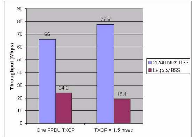
Fig. 7. Throughput of overlapping BSSs when TXOP is reduced.
