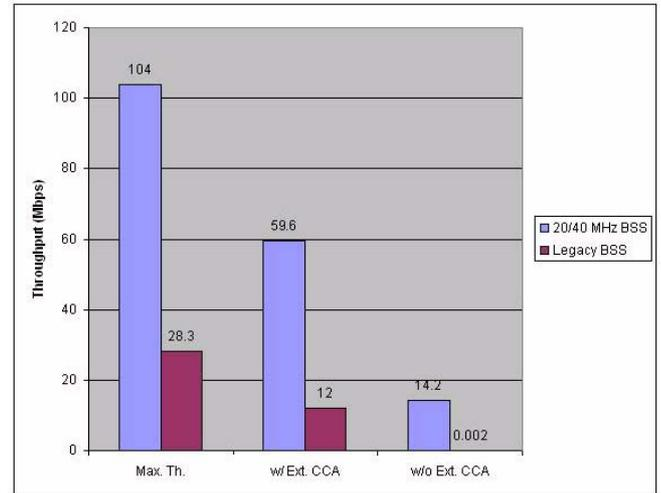
Fig. 4. Throughput of overlapping BSSs.
