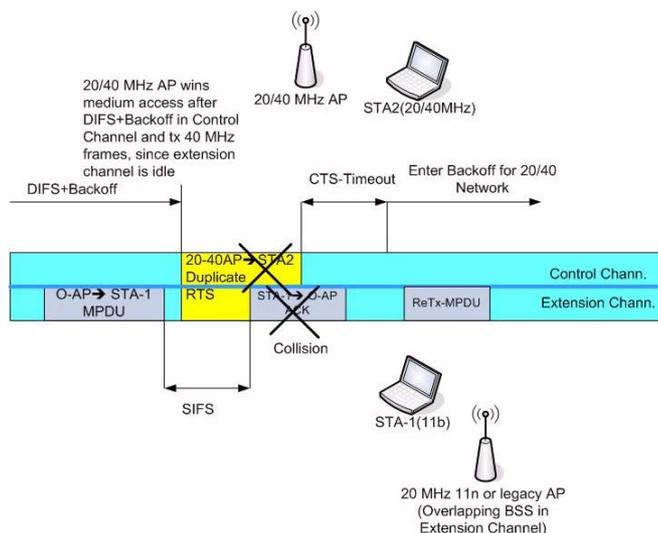
Fig. 2. Collisions in overlapping BSSs.
