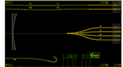
4ch x 25G LWDM Receiver Chip size: 7mm x 4mm
