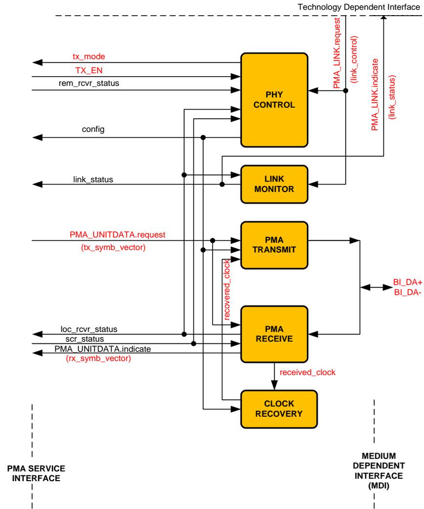
NOTE: The recovered\_clock shown indicates delivery of the recovered clock back to PMA TRANSMIT for loop timing.
