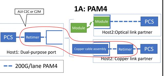
Short-reach copper cable channel may be enabled by low-loss designs or using retimers
