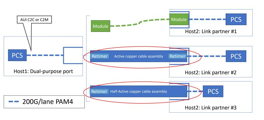
Copper Active cables allow the support of copper cables while architecture stays consistent with the optical PMD architecture
