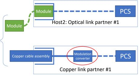
Optimize modulation independently for optical and copper PMDs
