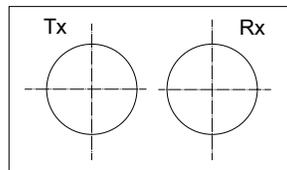
Figure 114–1—Example MDI receptacle (link segment side view)
