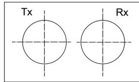
Figure 114–1—MDI receptacle (link segment side view)
