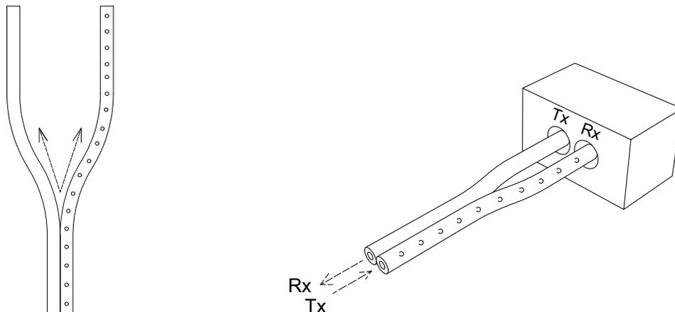
**Figure 114–2—Duplex POF cable splitting and connection to the 1000BASE-RHA MDI receptacle**
