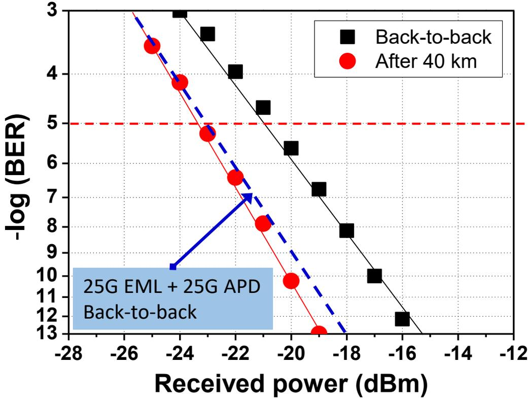
Target BER is  $5 \times 10^{-5}$  refereeing 25GBASE-LR in 802.3cc
