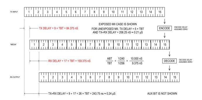
NOTE — TRANSFER UNIT TIME (UT) = NIBBLE TIME = FOUR BIT TIMES = 4 × ABT = 40 nS.
