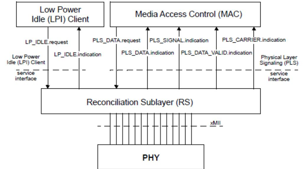
Figure 78-1—LPI Client and RS interlayer service interfaces
