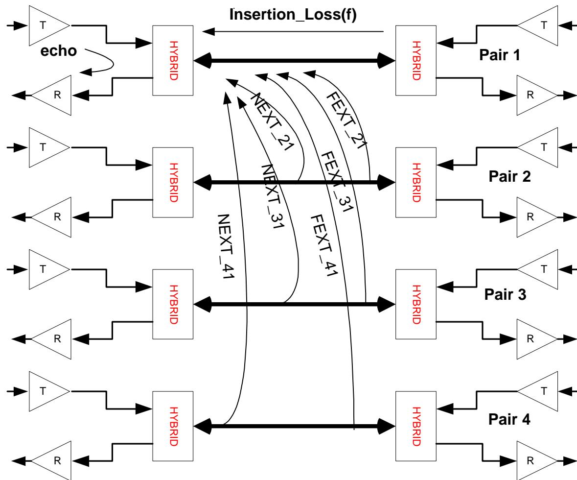
1000BASE-T uses DSP-based adaptive filtering to cancel the effects of echo, crosstalk and noise
