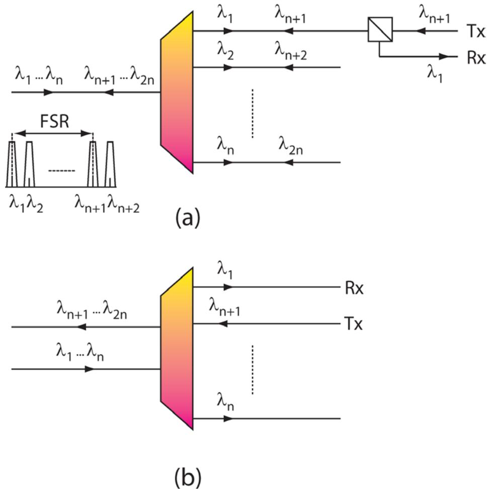
**Figure 56: RN with (a) Bidirectional, or (b) Unidirectional Transceiver at the ONU**
