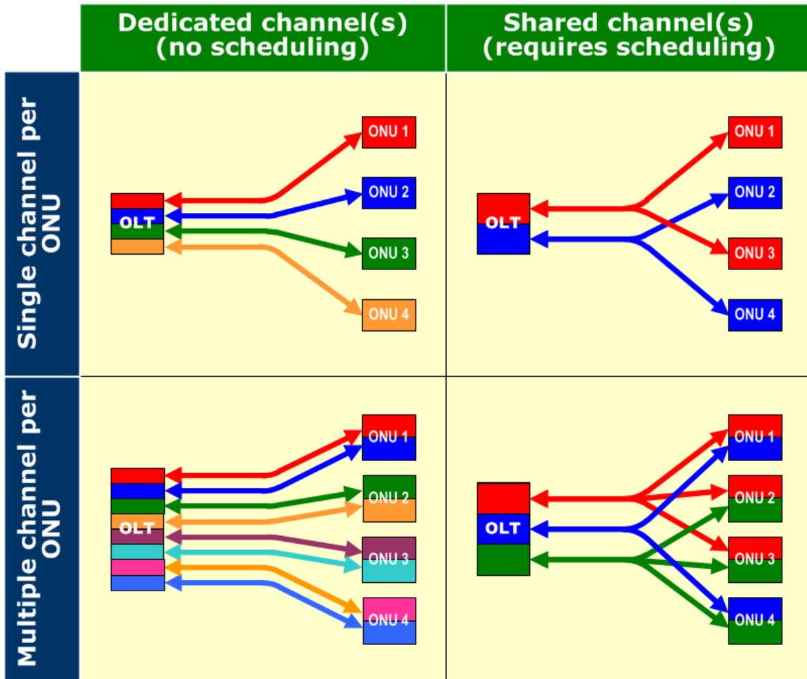
Note that each line connecting the OLT and an ONU represents a bidirectional channel consisting of one downstream wavelength and one upstream wavelength
