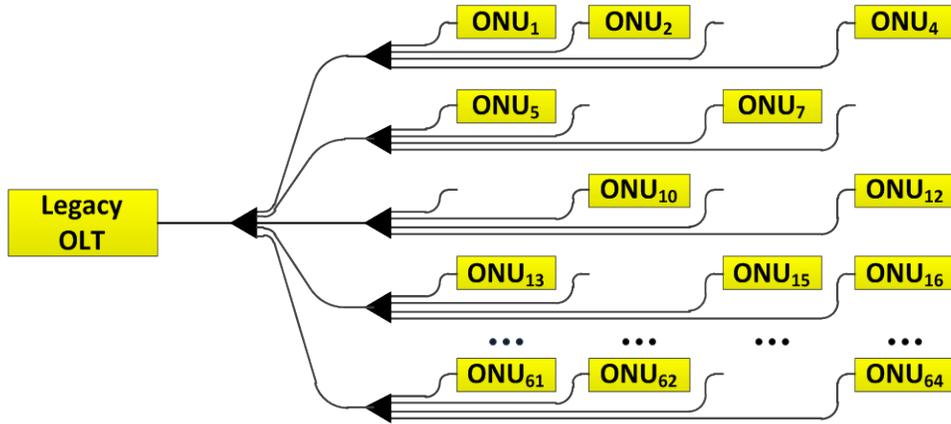
**Figure 24: EPON Access: Starting Point with 1G-EPON Devices**
