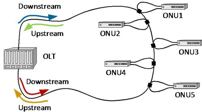
**Figure 8: Ring Topology using 2x2 Tap Couplers**
