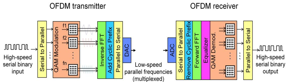
Figure 47: Base Electrical Physical Architecture of DD-OFDM
