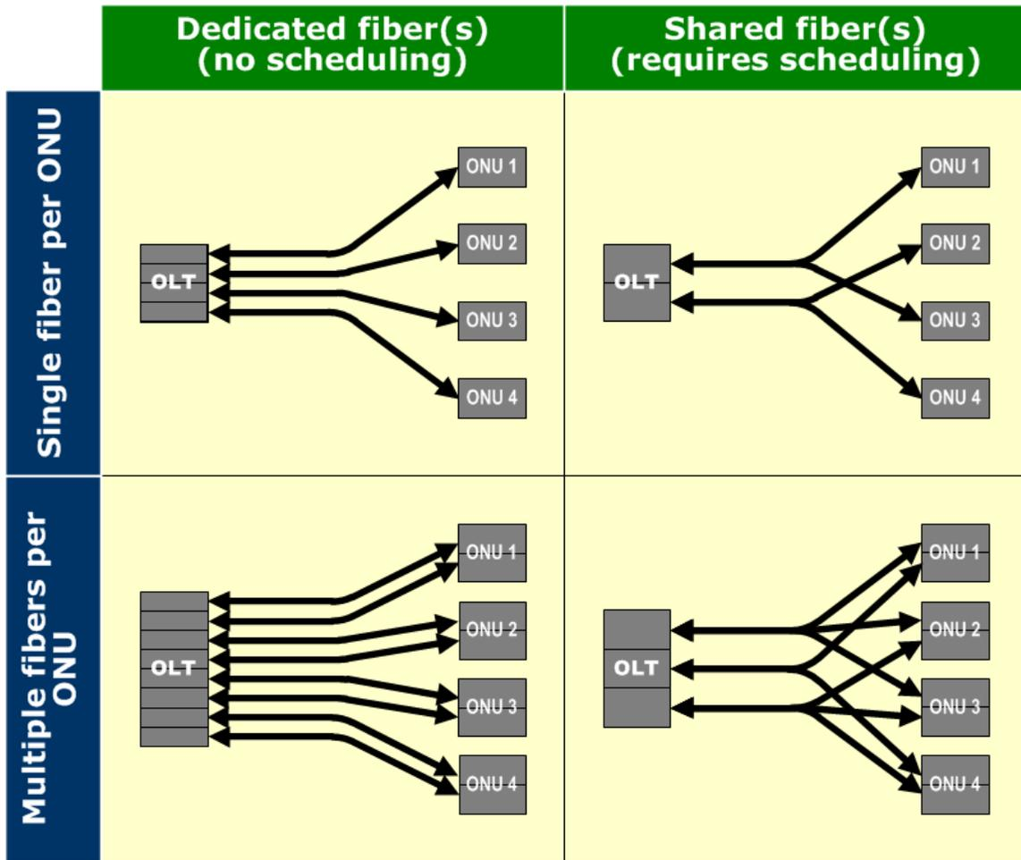
Note that each line connecting the OLT and an ONU represents a separate fiber (ODN)
