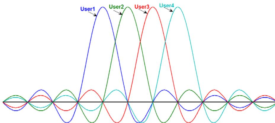
**Figure 49: OFDM Multiplexing**
