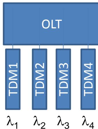
**Figure 38: MSD-WDM-PON with Multiple TDM domains [11]**
