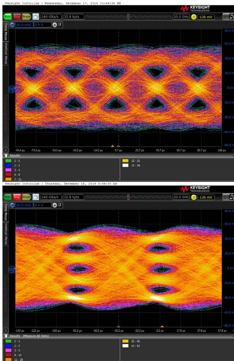
**Figure 45: Received Eye Diagrams (shown at -18 dBm) for Duobinary and for PAM-4**
