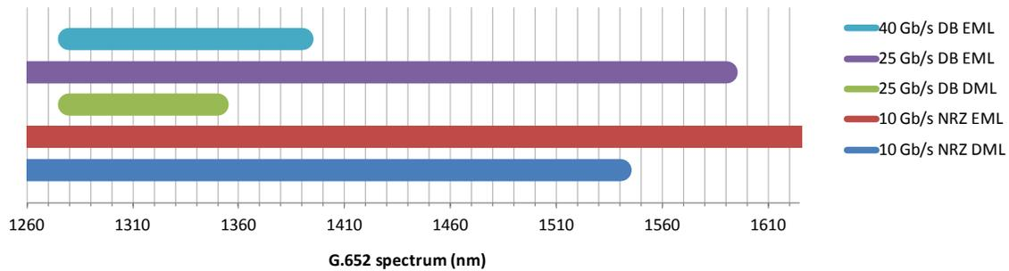
**Figure 43: Estimated usable SSMF spectrum (20 km) without DC**
