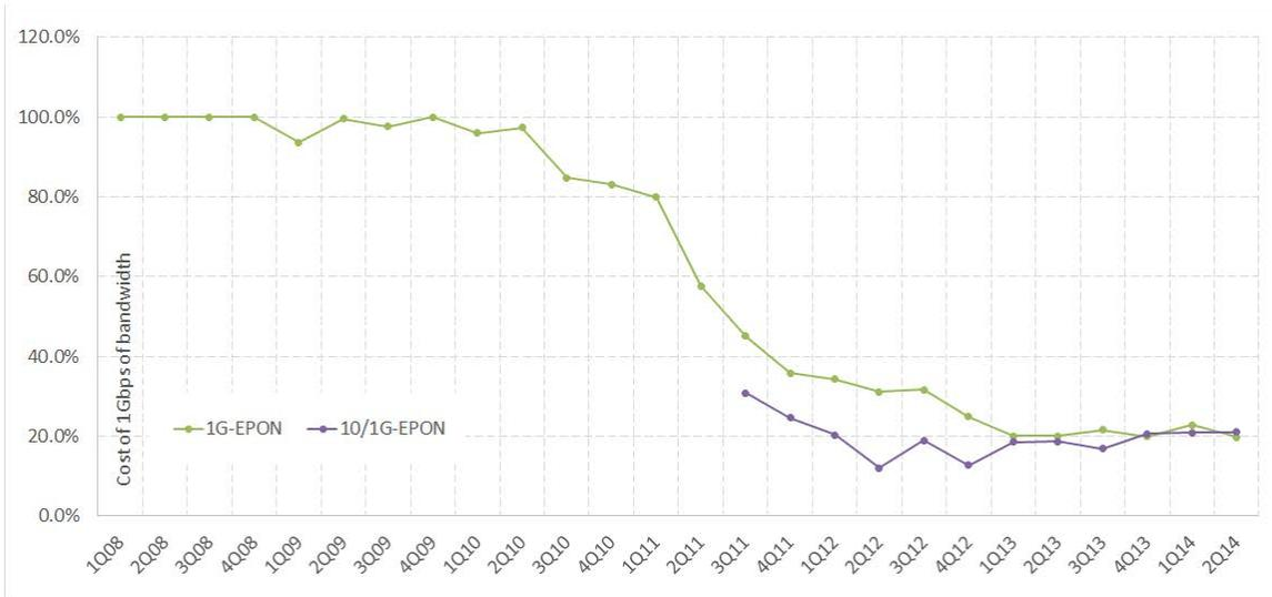
**Figure 67: Relative Cost for 1 Gb/s of Bandwidth**
