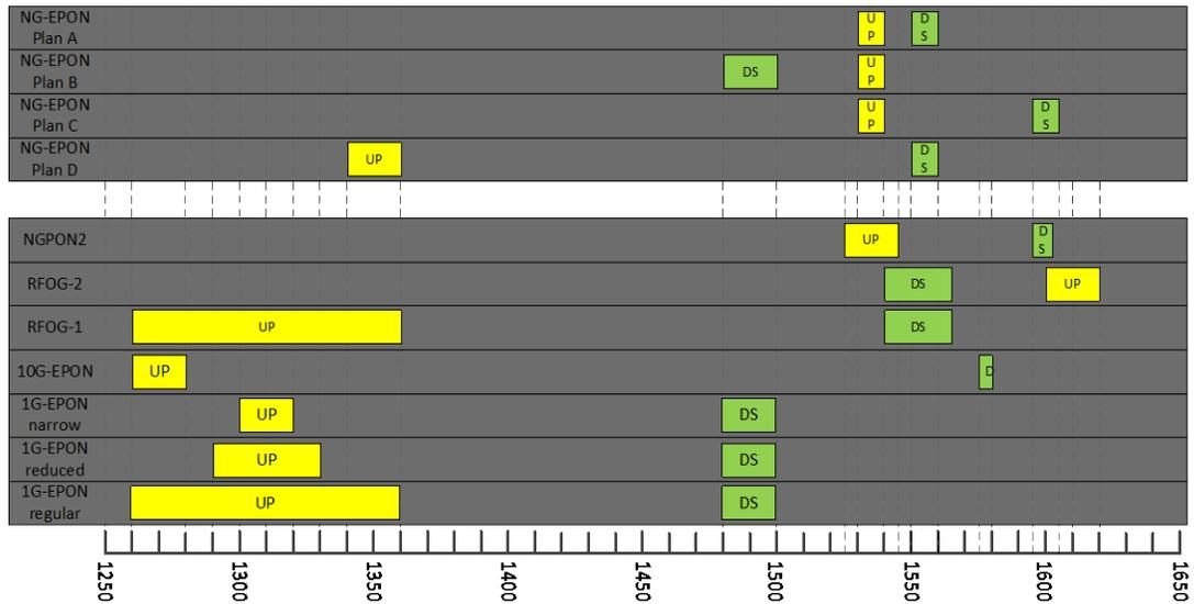
**Figure 57: Spectrum Allocation Bands for Optical Access Defined in IEEE Std 802.3, SCTE, and ITU-T**
