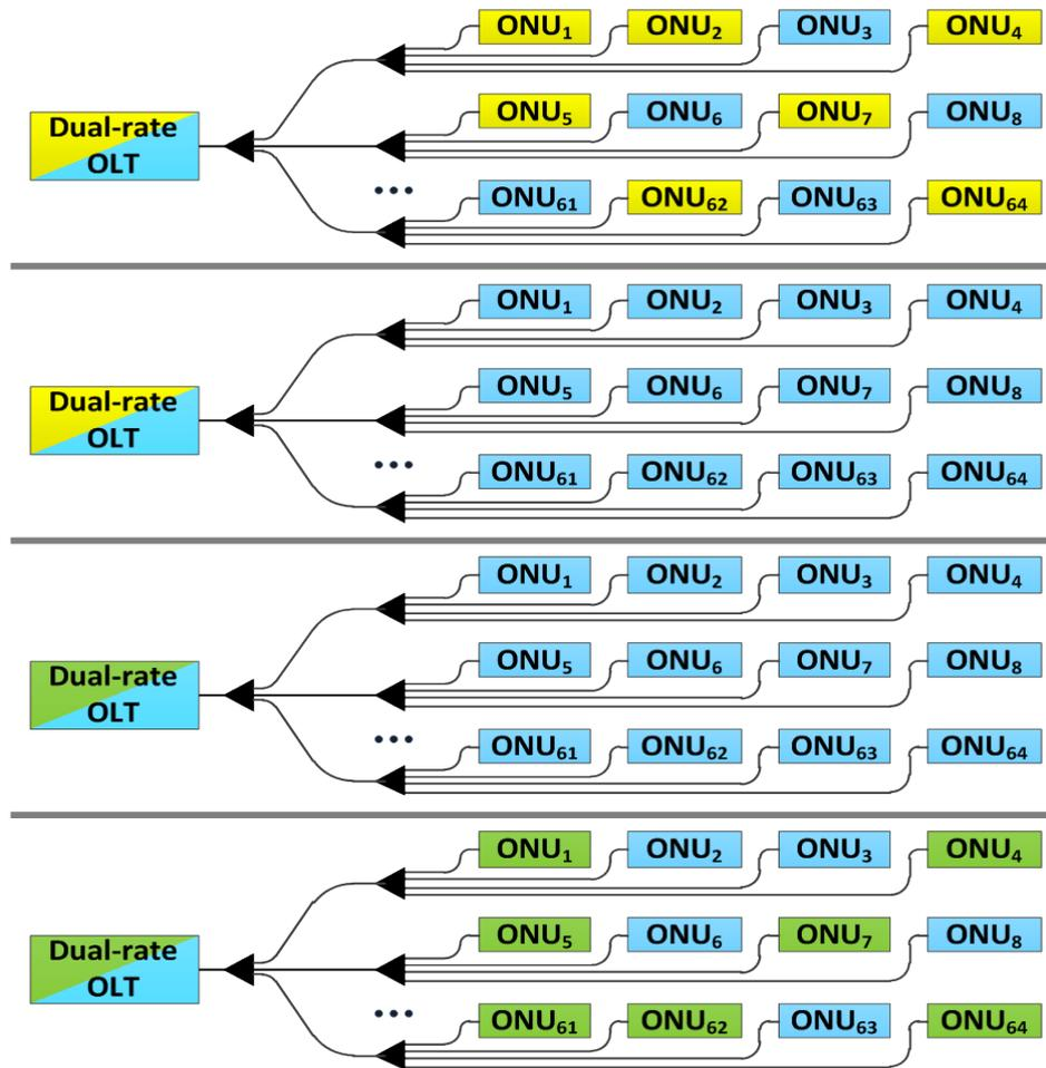
**Figure 29: Evolution from 1G-EPON and 10G-EPON Network to Two-Generation EPON Access**
