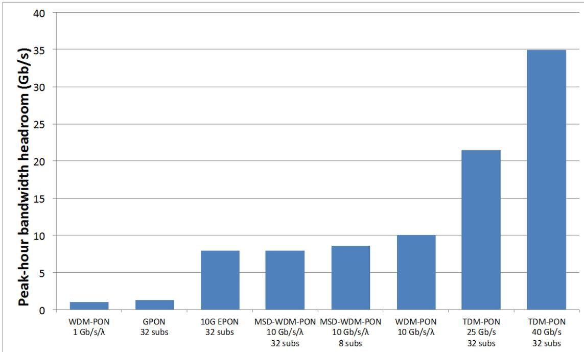
**Figure 21: Peak-hour downstream bandwidth headroom for FTTH**
