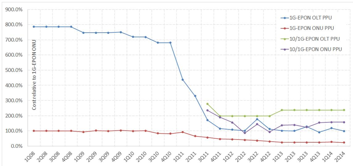
**Figure 66: Relative Cost of 1G-EPON and 10/1G-EPON ONU and OLT Devices over Time**
