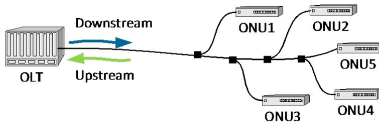
**Figure 7: Bus Topology using  $1 \times 2$  Tap Couplers**
