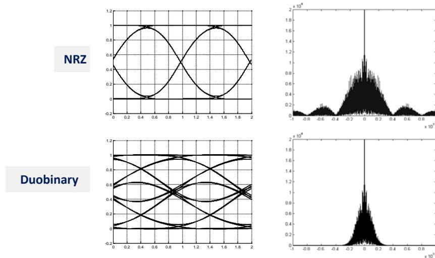
Figure 41: NRZ and Duobinary (LPF) Signals in the Time and Frequency Domains
