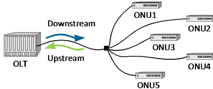
**Figure 6: Tree Topology using  $1 \times N$  Splitter**
