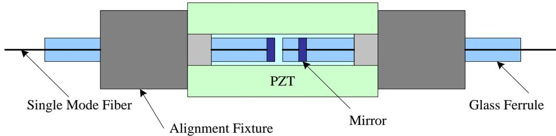
**Figure 63: Cavity length adjustment tunable filter**
