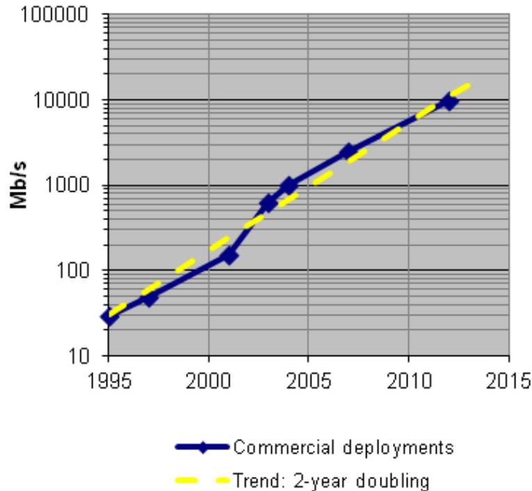
**Figure 36: Evolution of TDM-PON Downstream Data Rate**
