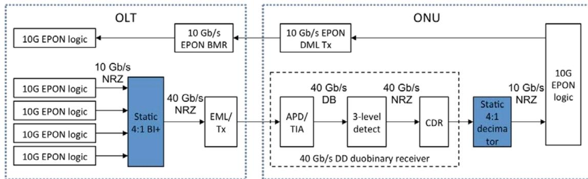
**Figure 37: Example of simple static bit-interleaved PON**
