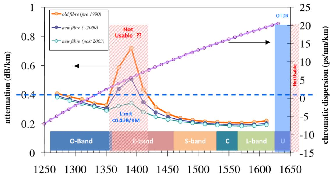
Figure 51: Attenuation and Chromatic Dispersion in Different Fiber Types [8]
