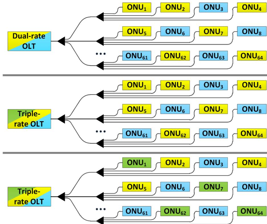
**Figure 28: Evolution from 1G-EPON and 10G-EPON Network to Three-Generation EPON Access**
