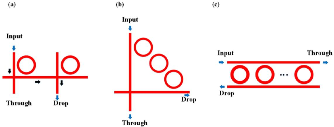
**Figure 62: Three topologies of micro ring tunable filters**
