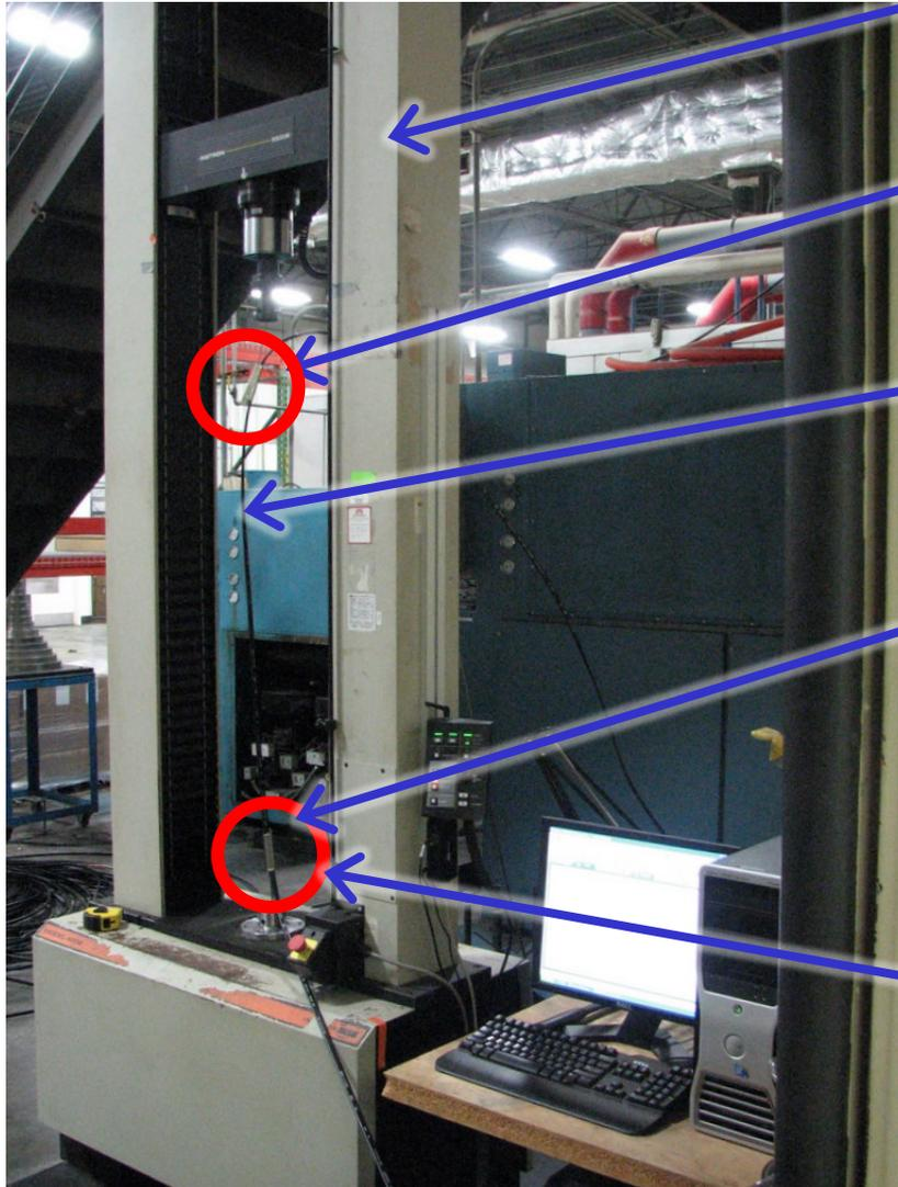
Instron Tensile Testing Machine
