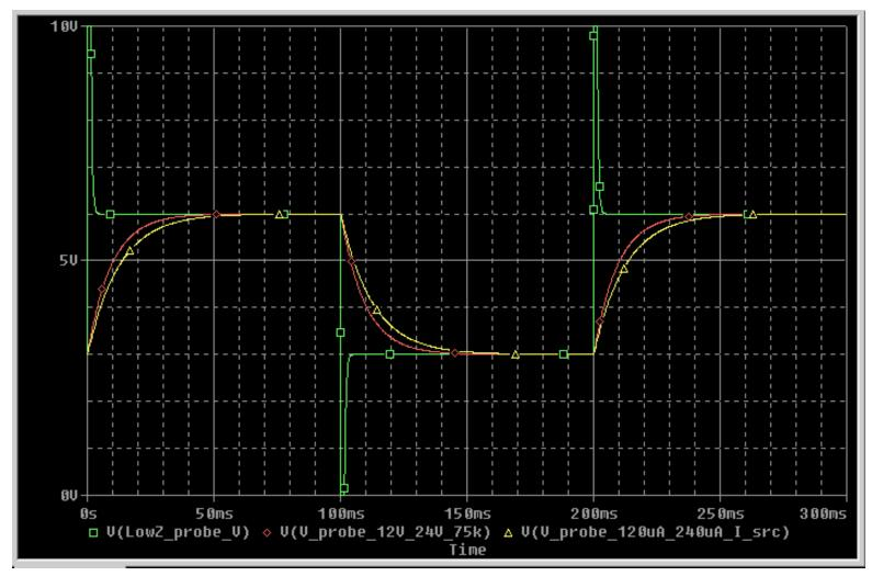
• 1% Settling Time Simulation Results, 500 nF Load Capacitance
