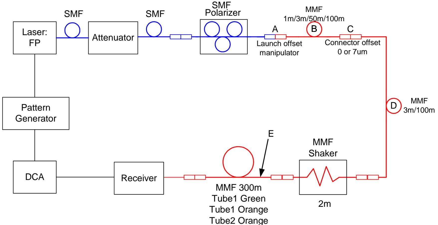
**When the shaker was used the measurements were also taken with the 0 or 7 um offset connector after the shaker. It was observed that it did not seem to matter where the connector was positioned.**
