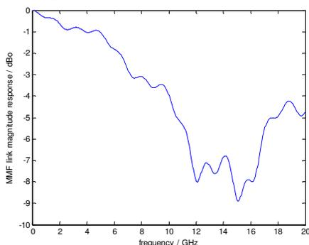
**Figure 1** An example of a MMF link magnitude response (contained in file **CamMMF1p2f108o23f.txt**).
