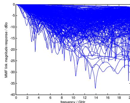
**Figure 2** Superposition of all 324 MMF link magnitude responses in this release.
