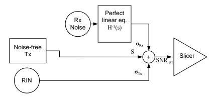
Where:  $\sigma_{Rx}$  is the receiver noise, *after* equalizer noise enhancement.
