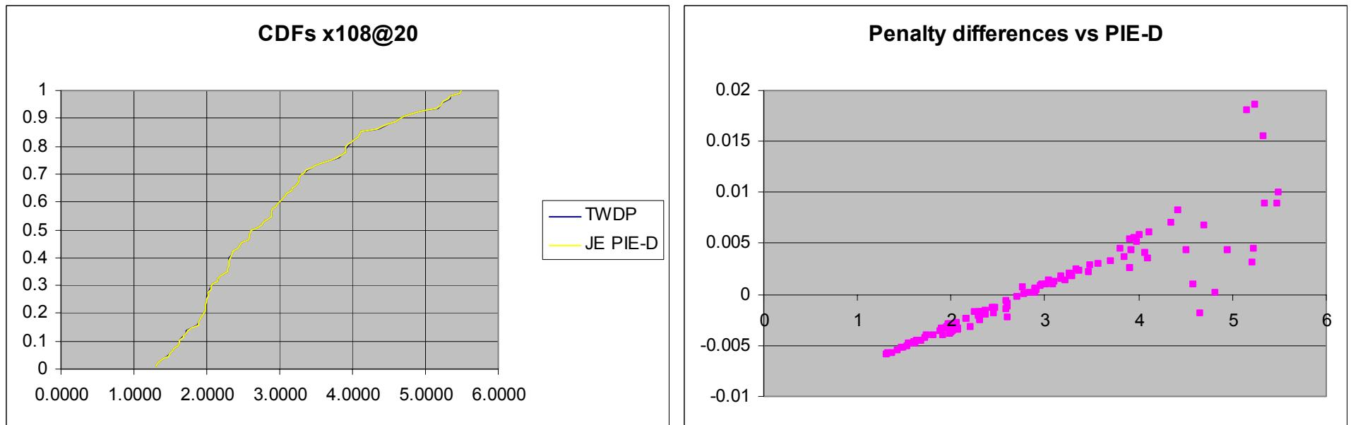
Within 0.02 dB; negative differences probably explained by round-off errors in PIE-D, simulated waveform, or elsewhere.
