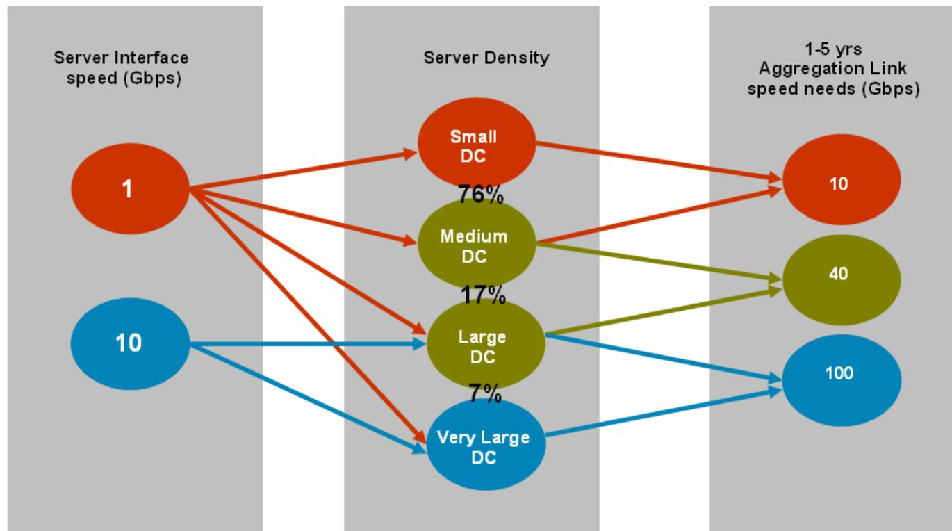
Different classes of Data Centers have different needs (and cost sensitivity) in terms of aggregation link speed.
