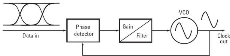
Low frequency jitter is transferred to the clock, high frequency jitter is not
