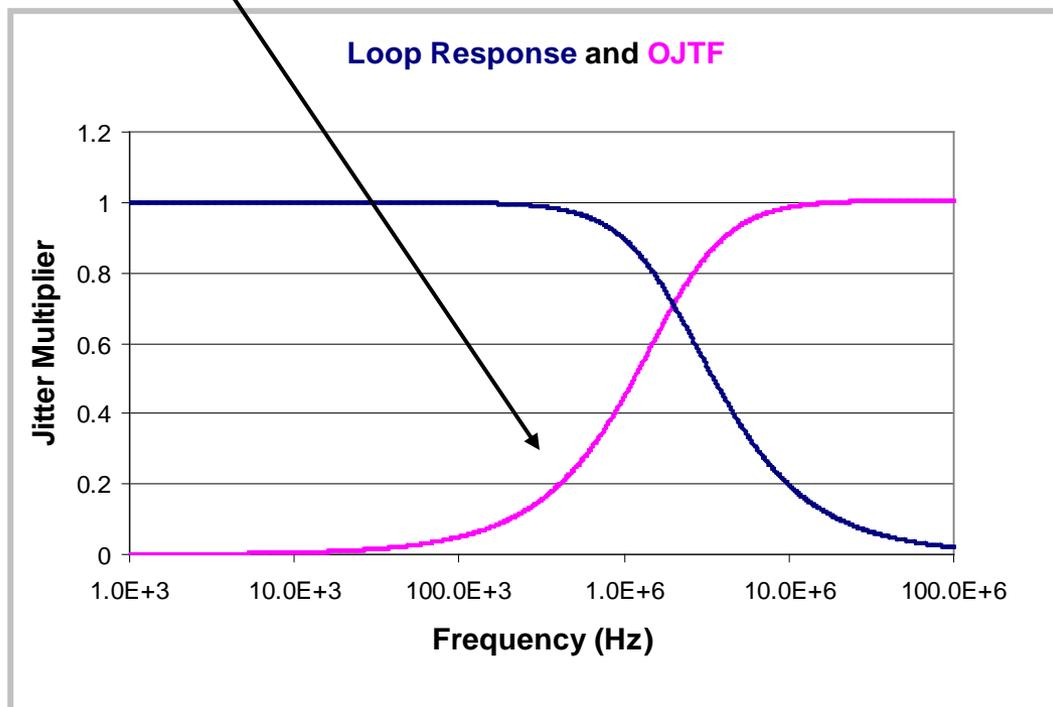
The observed jitter is a complement to the PLL jitter transfer response
