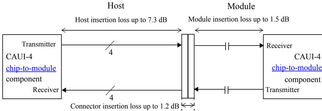
**Figure 83E-2—Chip-to-module insertion loss budget at 12.89 GHz**
