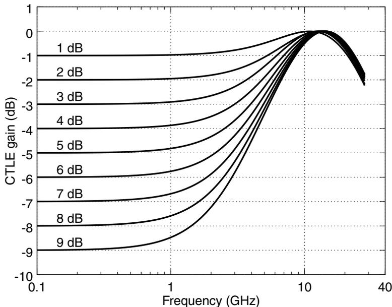
Figure 83E-10—Selectable continuous time linear equalizer (CTLE) characteristic
