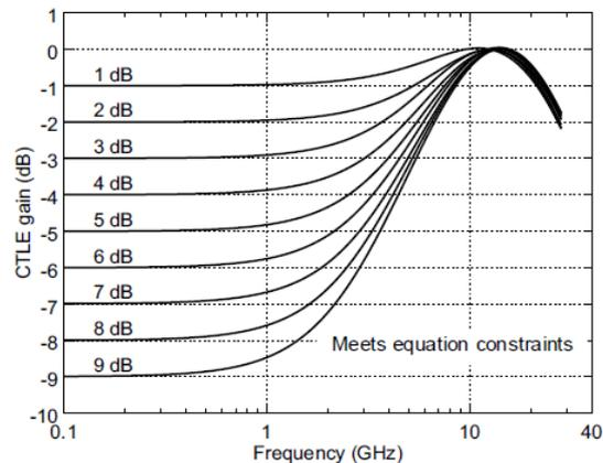
Figure 83D-11—Selectable continuous time linear equalizer (CTLE) characteristic
