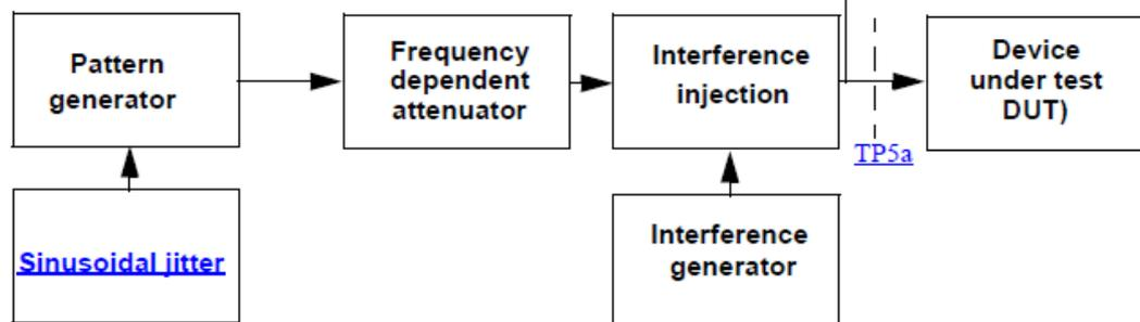
Figure 83D-12—Interference tolerance test setup
