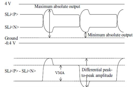
Figure 83A-5—Driver output voltage limits and definitions
