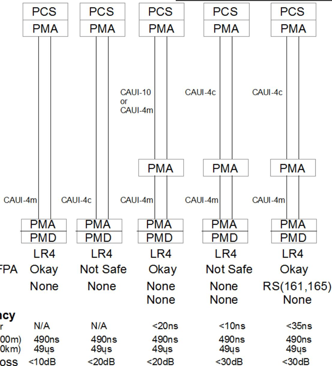
Host Loss derived assuming CAUI-4c2m is 10dB and CAUI-4c2c is 20dB
