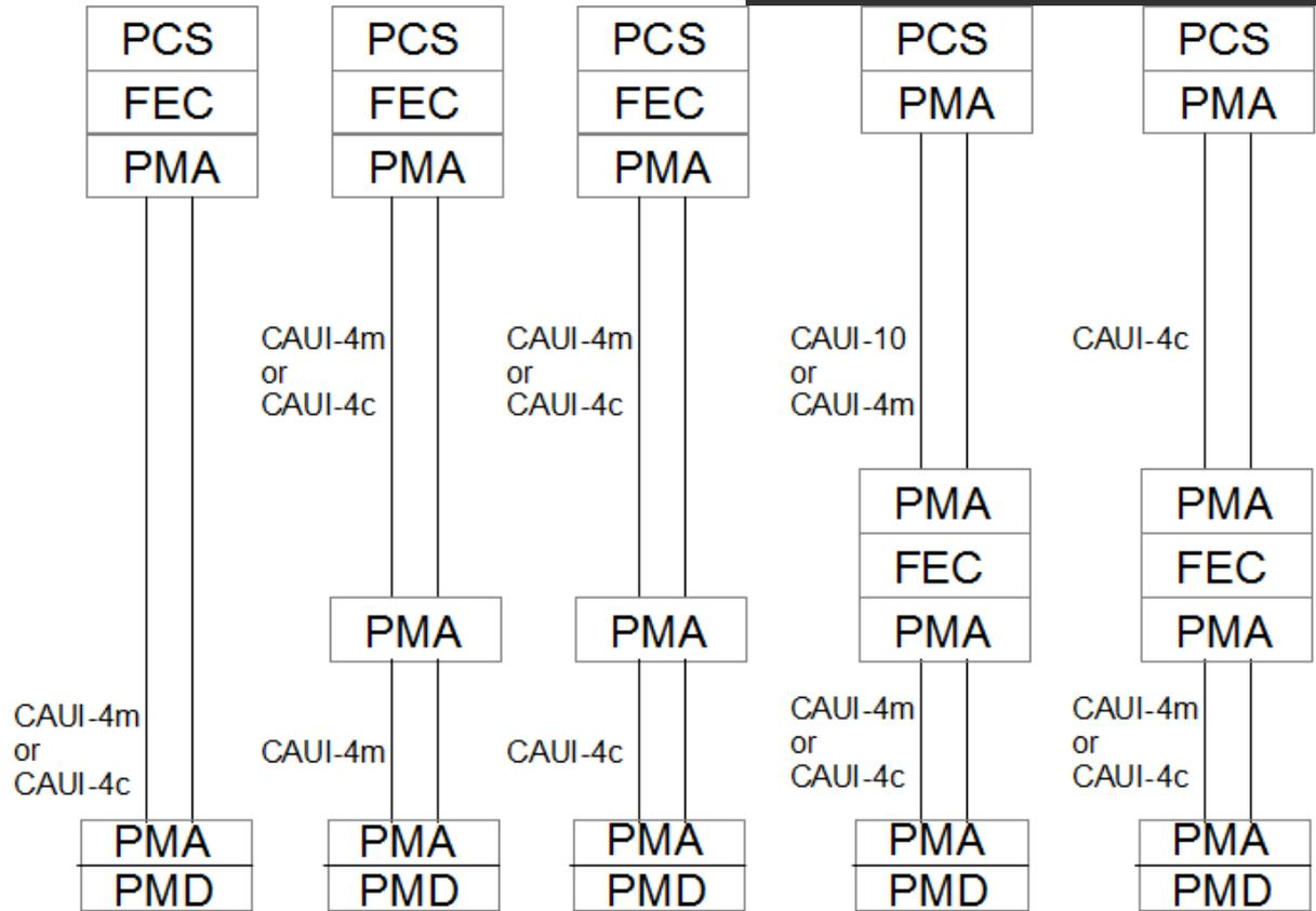
Re-timer latency derived from 120ns of RS-FEC latency + 30ns of 20 PCS lane alignment
