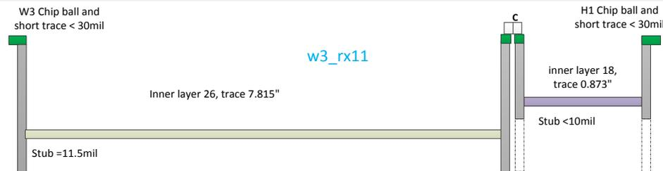
TUC872, with loss tangent 0.0078-0.0087. The differential pair is controlled at 92.50ohm with trace width about 4.5mil and core thickness 4 mil.
