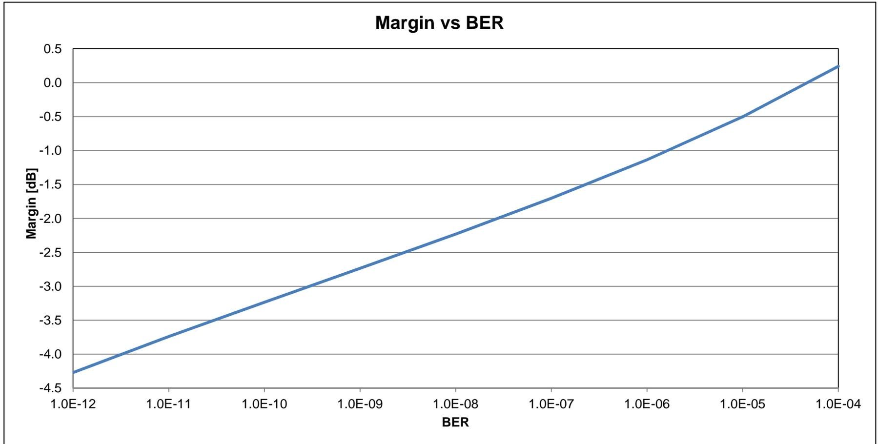
The above chart shows the benefit to an optical link from FEC. Operating at a higher BER not only appears to improve the Rx sensitivity but all the noise related penalties are reduced as is the power required to open the eye to a target width. For 100G PSM4, capturing all the benefit of KR4 FEC enhances the link margin by ~4.3 dB when compared to operating at a BER =  $10^{-12}$  without FEC.
