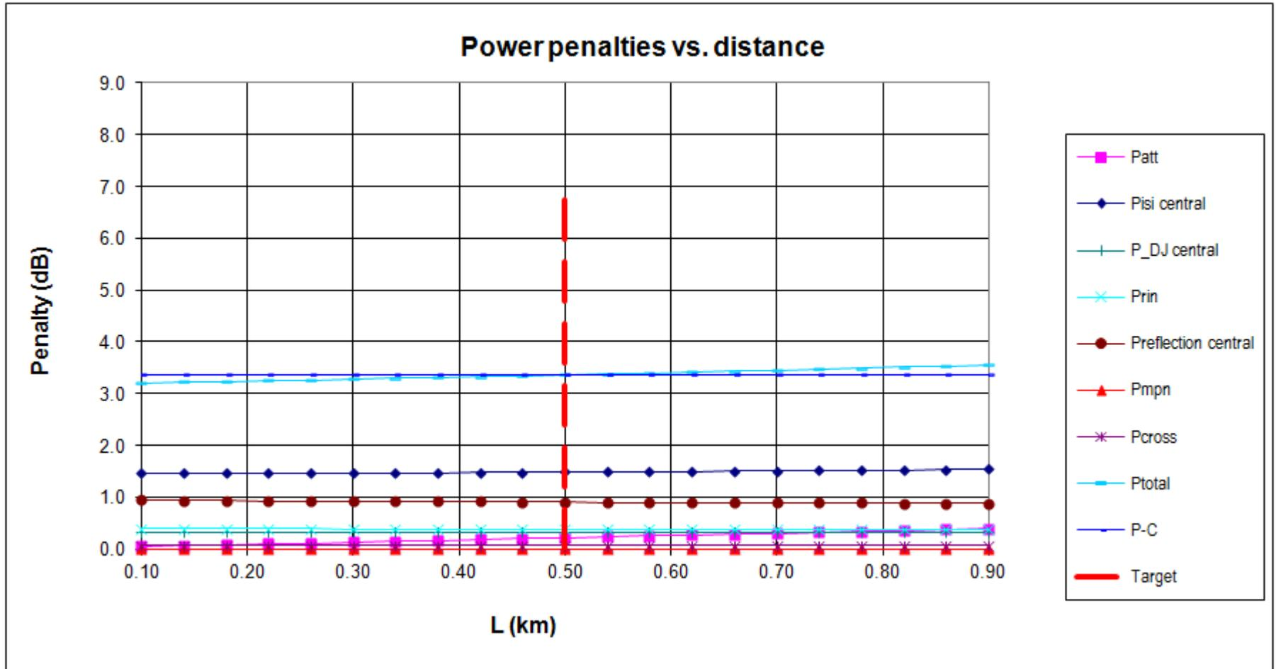
The above chart is taken from the tab Base of the updated Example PSM Link Model. It does not explicitly show the power required for the target TP4 eye opening,  $P_{eye}$ , but distributes the penalty in other power penalties. For this example,  $P_{eye}$  at 500 m equals 0.38 dB.
