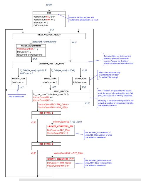
In **red** the change due to de-rating from the original chart – final format and proper rounding can be defined once know PHY parameters
