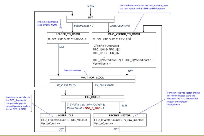
The same state diagram (see wbove) can be reused with proper changes of FIFO\_II\_SIZE:
