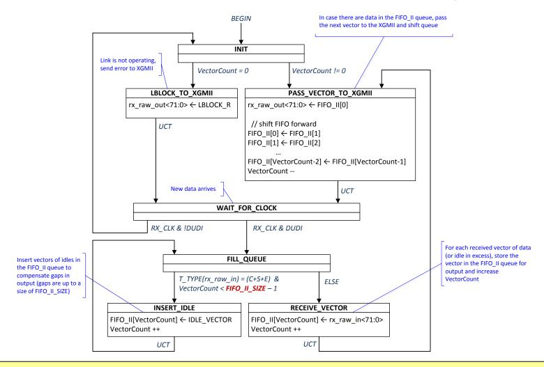
The same state diagram (see above) can be reused with proper changes of FIFO\_II\_SIZE:
