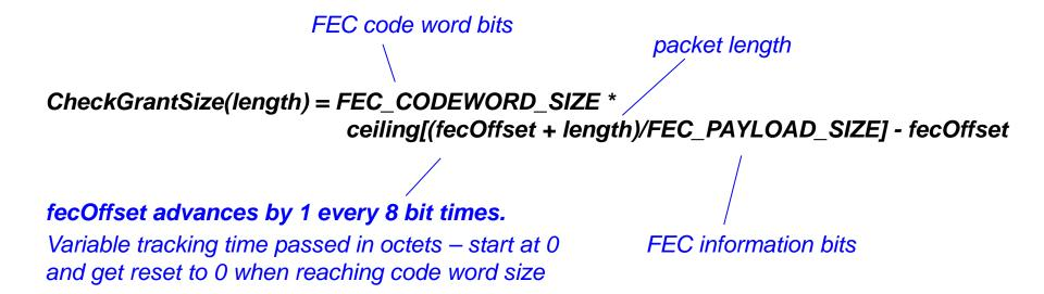
The function returns the future time at which the transmission of the current frame (including FEC parity overhead) is completed - when the cumulated data (tracked by the variable *fecOffset*) exceeds the FEC\_PAYLOAD\_SIZE, a new FEC Code Word is started
