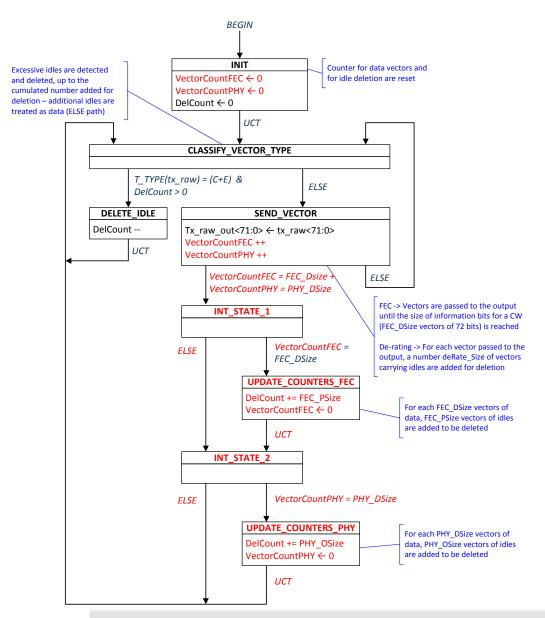
In **red** the change due to de-rating from the original chart – final format and proper rounding can be defined once know PHY parameters
