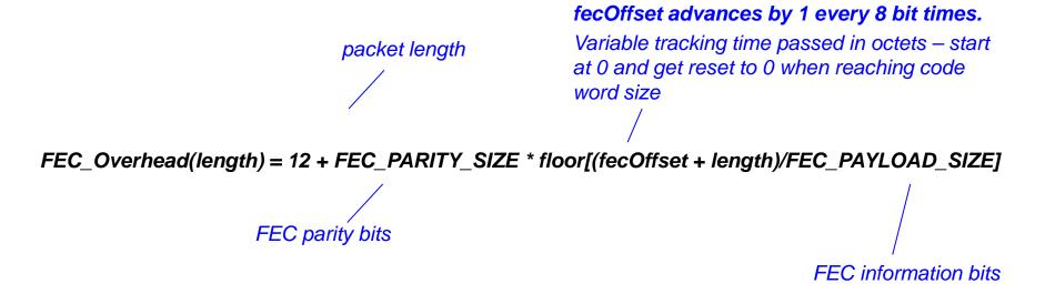
The function returns the length of the data to transmit and cumulates information bits (tracked by the variable *fecOffset*) - when the cumulated data exceeds the FEC\_PAYLOAD\_SIZE, a FEC\_PARITY\_SIZE interval is also included to space for parity
