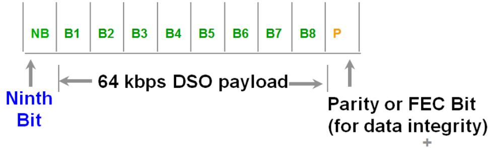
8 Payload bits + NBS + Parity bit = 10 bit DSO format
