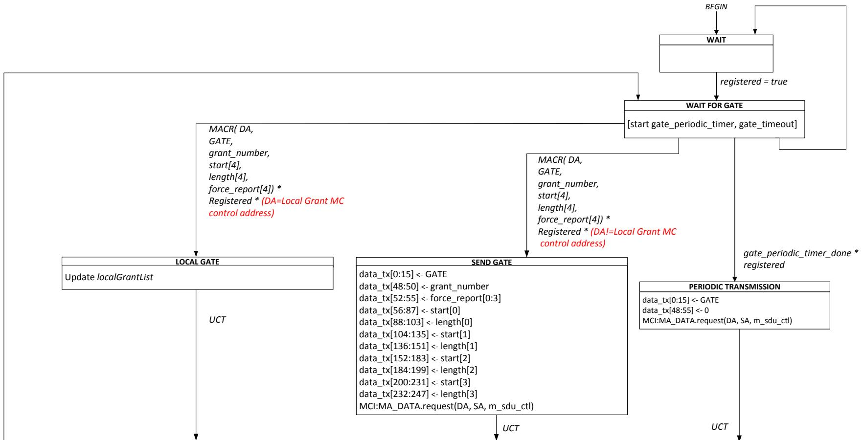
Definition of new MAC control multicast address ( e.g. 01-80-C2-00-00-02) and extension of the `MA_CONTROL.request` primitive
