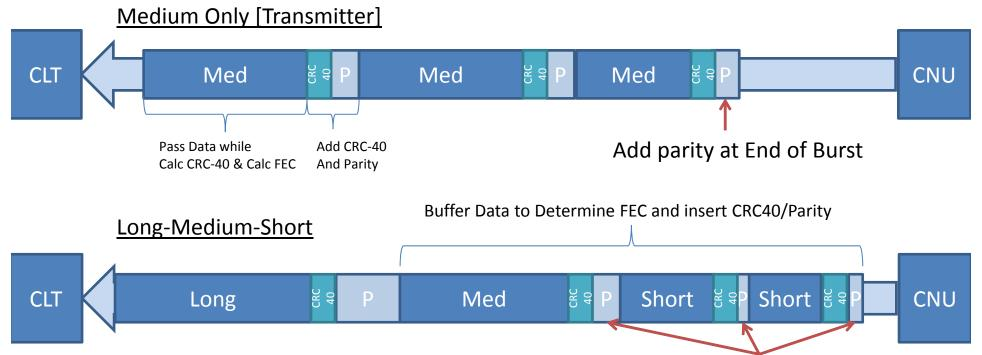
Example: Insert 3 parities at End of Burst End of FEC blocks.
