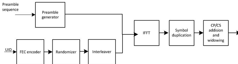
**Figure 7-25 - Fine Ranging Transmitter Processing**
