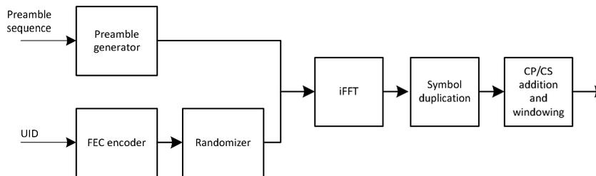
**Figure 7-20 - Block Diagram of Initial Ranging Transmitter Processing**
