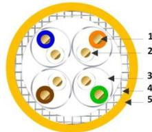
1800MHz S/FTP AWG22 / OD = 8.3mm
