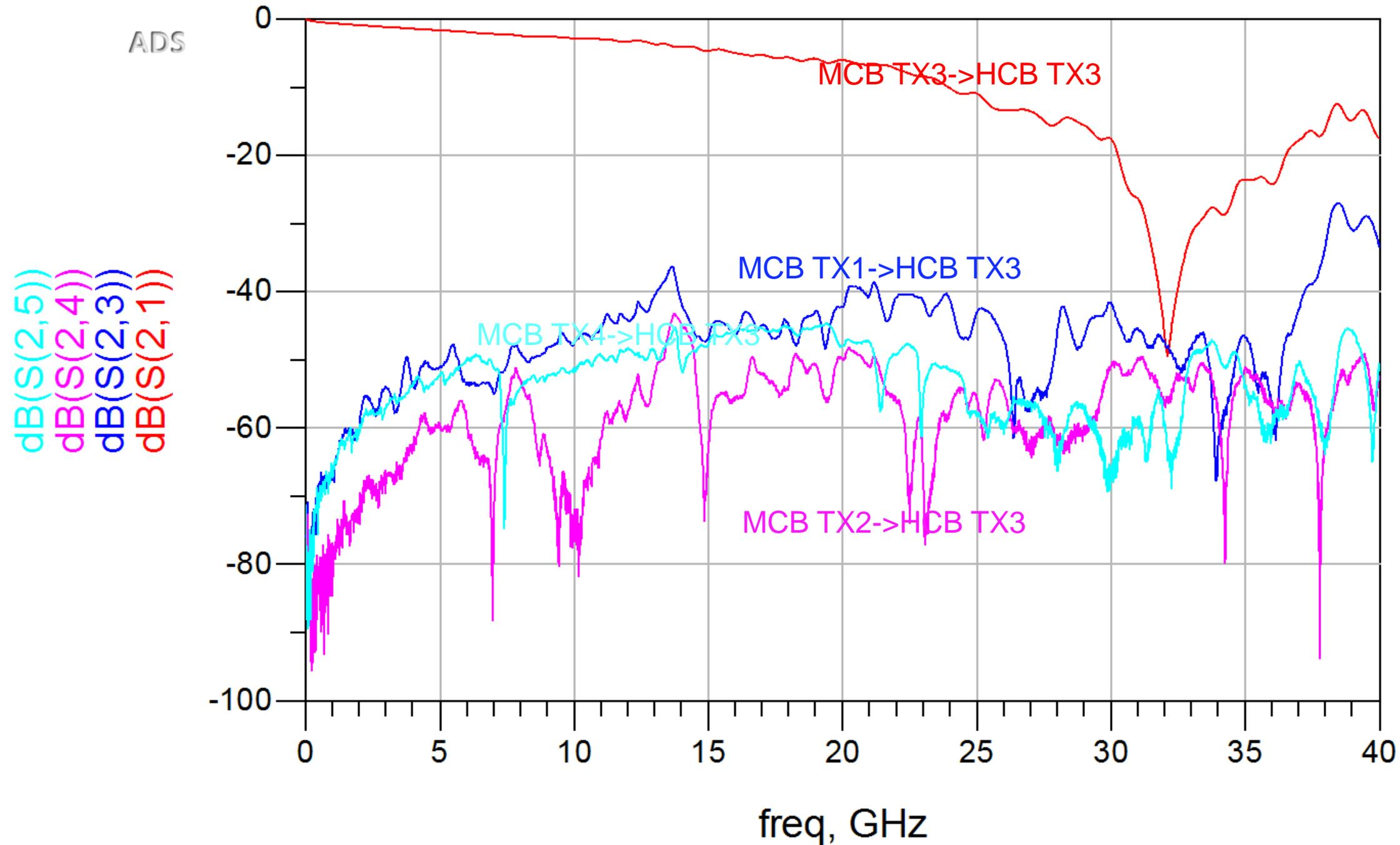
FEXT measured per procedure for mated test boards =2.7mV rms.
